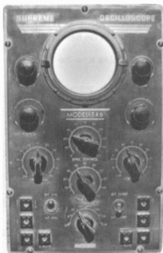
SUPREME MODEL 546 – This 1930s vintage oscilloscope features a brass front and an oak cabinet. (John Schehrer – Joplin, MO)
