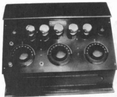
JOSEPH W. JONES BATTERY SET – This TRF set, ca. 1924, has 5 exposed tubes, plus the usual 3-dial tuning arrangement. (Larry Chestnut – Ellington, CT)
