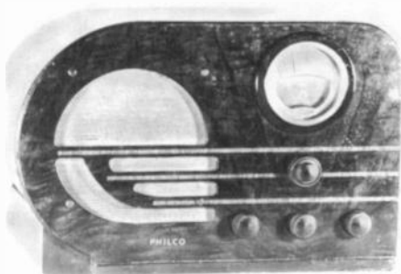
PHILCO MODEL 38-10 – This 1938 standard broadcast and shortwave receiver has a walnut veneer cabinet with photofinishing on the front panel. (Robert Bailey – Jacksonville, FL)
