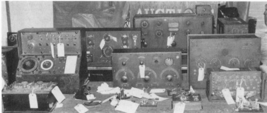
Left to right, the larger pictured items are a British Marconi Direction Finder Type 11, a Canadian Marconi Type 2843, an American Marconi Type 122 (or 119 or 120), an American Marconi Type 101, a Wireless Specialty Apparatus Co. IP-77, and a British Marconi Type 55 amplifier. These six items alone brought $97,800.
