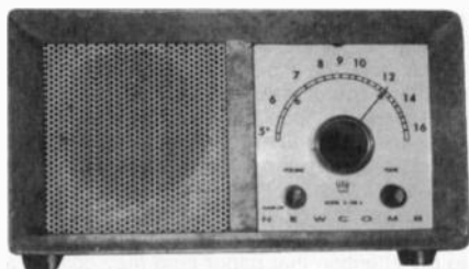
NEWCOMB MODEL B-100A – This simply designed AC/DC radio was made by a West Coast manufacturer of well known audio amplifiers. The chassis uses a combination of miniature and octal tubes. The cabinet has a leatherette covering. (Harry Pawowaruk – St. Cloud, MN)
