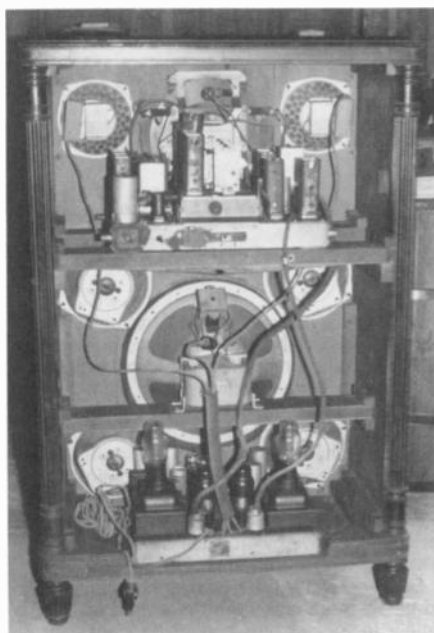
Figure 3. This cabinet has to be rugged to withstand the combined weight of the receiver chassis, 3 speakers, 4 resonators, and the power unit chassis. Not surprisingly, Rider's Volume VIII, page 39, gives instructions for removing the cabinet top and adjusting the door hardware.
