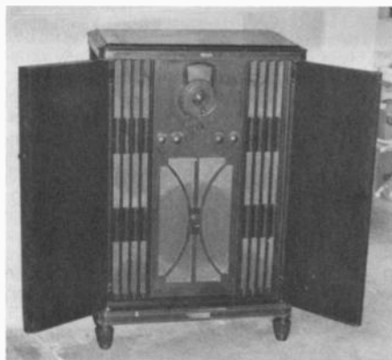
Figure 2. Note the 7 speaker grilles and the automatic tuning dial. There are 6 controls — Tuning, Off-On/Bass, Magnetic Tuning, Band Switch, Volume, and Treble/Selectivity.
