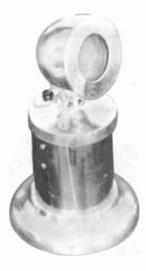
MICROPHONE MODEL UNKNOWN – This attractive 10½" high brass and nickel-plated microphone is probably from the 1920s. It has a 5-prong connector socket in the back and an inverted 4-prong "Pilot USA" tube socket in the base (for a Type 864?). The only other identified parts are a rectangular, metal-clad condenser stamped "Made in Germany" and three "Arthur H. Syuch" grid-leak type resistors, all in the base. It is possible that this may be a prototype. (Bill Ross – Winnetka, IL)
