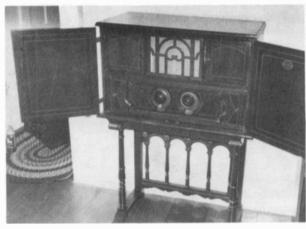
Figure 2. The Atwater Kent 40 with the Pooley 7500 cabinet doors open.
