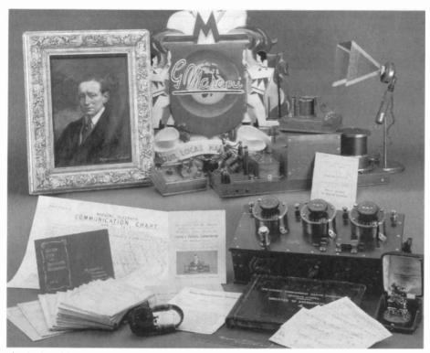
A selection of the items include a dealer sign, a multiple tuner, a coherer receiver, and Melba's microphone.
