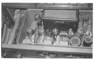
Figure 5. The sliding drawer gives easy access for tube testing and for measuring power supply voltages. The power supply terminals are accessible when the power supply lid is removed.
