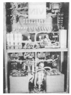
Figure 2. A rear view of the Weston tube tester shows the "iron" that makes the unit weigh 130 pounds!
