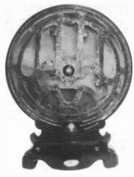
BORKMAN RADIO CORP. MODEL 18 – Also known as "The Chinese Cone-Flex," this unusual speaker resembles a cone-type speaker, but consists of a papier-mâché horn facing the side. The driver is located in the base. The speaker is 19" high. (Ed Bell – Raleigh, NC)
