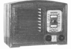
**EMERSON MODEL UNKNOWN** – This radio has a typical mid-1940s tube lineup and Emerson chassis design. The unique thing about this set is its cabinet construction, which is made of cardboard covered with a textured contact-type paper. (*Mike Keller – Columbus*, *OH*)
