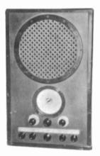
RCA MODEL AVR-5 – This 1934 communications receiver has 9 tubes, AF and RF gain controls, a CW oscillator, and a 10" speaker. It receives 150 Kc to 18 Mc. The unusual wooden tombstone-style cabinet stands 22" high. (Frank Franowsky – Santa Fe, NM)
