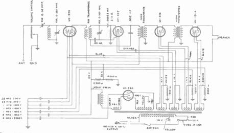
Figure 5. The Polydyne Models Q15 and Q16 schematic. Note the five separate filament windings on the power transformer.
