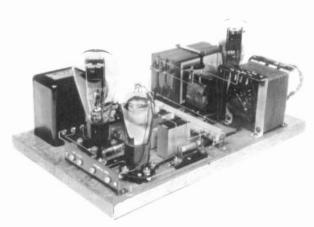
LOFTIN-WHITE HOME BREW DIRECT-COUPLED AMPLIFIER – The only way to find out how the Loftin-White direct-coupled amplifier sounds is to build one from the company's 1930 plans and try it. The iron is all Silver-Marshall, and aside from new capacitors in the old filter cans, everything is from the period. It works all right, but the hum level is atrociously high. Anybody have an Electrad L-W kit? (Alan S. Douglas – Pocasset, MA)
