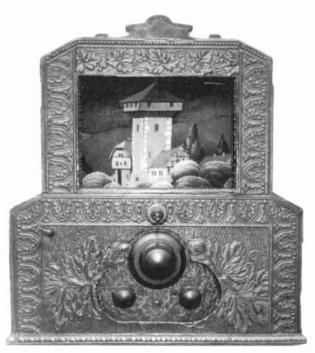
Figure 1. A front view of the ornate Polydyne. Note the dial lamp above the tuning dial. The toggle switch centered between the two control knobs is the radio's on/off switch. A full color print of this same radio appears on the inside back cover!
