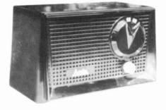
**ARVIN MODEL 950-T2** – This is an inexpensive, 5-tube, AC/DC broadcast receiver. Manufactured in 1958, this radio is a prime example of "Rocket Age" styling. Notice the novel way that the tuning knob uncovers only the dial scale numbers being tuned, while covering all the others (*Robert Bailey – Jacksonville, FL*)
