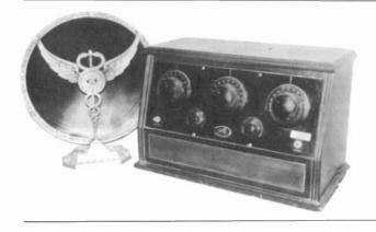
PATHÉ MODEL U5 AND PATHÉ SPEAKER, GRE-CIAN MODEL – Made by Pathé Phonograph and Radio Corp., this 5-tube, 3dial set uses either storage battery tubes or McCullough AC tubes. (Wally Worth – Wollaston, MA)
