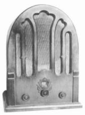
SHARP MODEL 30 – This small, 3-tube cathedral, only 14\* high, made in Japan, has a veneer cabinet with a wooden back cover. Its tube complement consists of Types UY4-56, 12A, and 12F. It also has a fine-tuning control. (*R. Suslovich – McLean, VA*)
