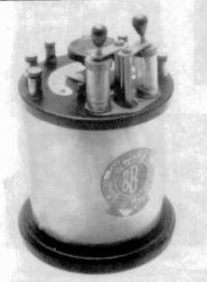
CLYDELCO CRYSTAL SET – This double glass-enclosed catwhisker and galena crystal set was manufactured by the Clyde Electrical Co. in 1923. The tuning variometer, enclosed in celluloid below the top panel, has the GPO (Government Post Office Approval) No. 871. It is one of my most interesting crystal sets from Great Britain. (Erwin Macho – Vienna, Austria)
