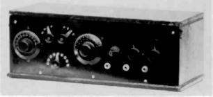
Figure 5. The 3-tube Reinartz receiver.
