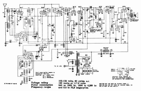
Figure 3. Schematic of the 1938 Emerson Model X183, showing the 15-tube circuit.
