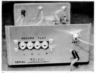
Figure 3. A rear view with all connectors shown. The grounding stud is located at the lower right of the RCA-type jack strip.
