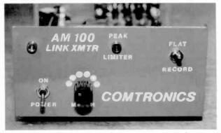
Figure 2. All operating controls and indicators are located on the front panel. 20
