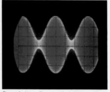
Figure 5. An oscilloscope display of the RF output. The 800 kHz carrier is amplitude modulated by a 1 kHz audio signal at about 80%.
