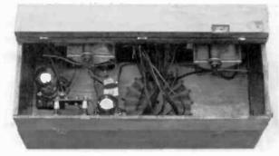
Figure 4. The interior of a 2-tube Reinartz receiver.
