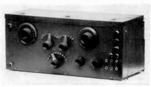
Figure 3. The 2-tube Reinartz receiver.
