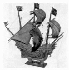
Figure 1. This ship cone speaker, a model of the Santa Maria with its middle mast used as a paper cone, was produced as a kit by Miniature Ship Models, Inc., of Philadelphia, PA.
