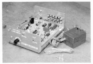
Figure 1. The AM-100 with its cover removed, along with the plug-in DC power supply and wire antenna in its rolled up state.
