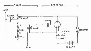
Figure 1. The Reinartz receiver circuit.
