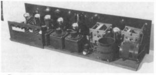
Figure 8. The rear view of the restored Tropadyne receiver chassis.
