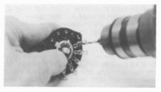
Figure 4. A drill bit slightly larger than the inner diameter of the eyelet can be used to remove the flared end of the eyelet. In this photograph, an electric hand-drill is used to drill out an eyelet.
