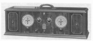
Figure 1. The AR-812, manufactured in 1924, was the first commercial superhet. The handle on this set qualifies it as a "portable."
