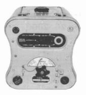
MAE WEST EMERGENCY RADIO – Manufactured by Kingston Products Co. of Kokomo, Indiana, this unit was used by downed World War II pilots to call for help. The odd shape was to fit the user's knees while he turned a crank to generate power. (Clark Trissell – Lincoln, NE)
