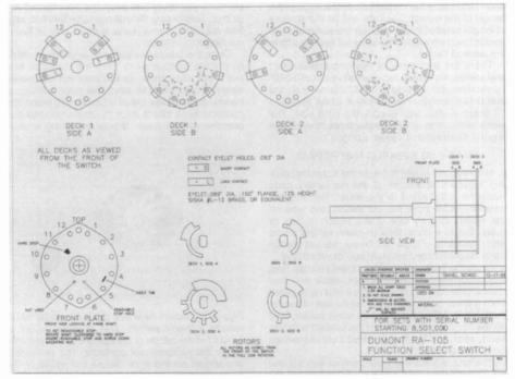
Figure 2. An example of complete mechanical documentation of the old switch.
