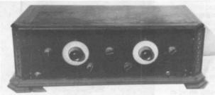
Figure 9. The panel view of the Victoreen superheterodyne receiver.
