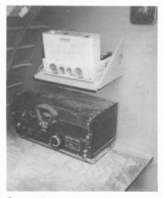
Figure 2. The radio compartment in the B-17 bomber was on the forward left side of the airplane. The BC-348H receiver shown here is mounted on a shock mount but is not functional. Above the receiver is a BC-456 modulator which is part of the SCR-274-N Command set. This photo was taken aboard the B-17 "Nine-O-Nine" which is owned by the Collings Foundation of Stow, Massachusetts.
