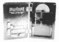
HELIPHONE CRYSTAL SET – This U.S. crystal set was manufactured by Garod (Gardner-Rodman Corporation) and was first advertised in July 1922. The tuning is accomplished with sliding flat coils and an open catwhisker/galena detector. The two hinged panels are constructed of wood. (Erwin Macho – Vienna, Austria)
