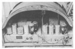
Figure 2. Rear view of the Pilot Model 40174 "All-Wave" receiver showing both chassis.
