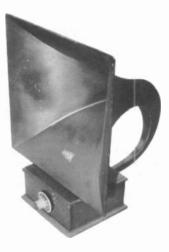
CALLOPHONE HORN SPEAKER – The huge metal horn bell on this speaker measures 15" square. The driver inside the rear of the wooden box is adjusted for tone by the front dial which has a long shaft to the driver. Manufactured by the Callophone Co. of New York City, it sold for \$35 in 1924. (Dave Crocker – Mashpee, MA)
