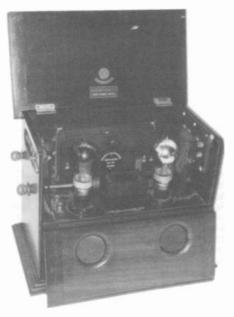
MARCONIPHONE V2A – Found in mint condition, this 2-tube, reflex, long-range model receiver was manufactured in 1924. It operates on the 300-390 meter wavelength. (*Jim Taylor Bournemouth*, *England*)
