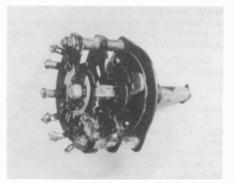
Figure 1. This typical phenolic rotary wafer switch exhibits extensive damage. Note the broken wafers.
