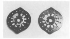
Figure 7. When rebuilding wafer switches, it is necessary to install the rotors before the stationary contacts are installed. This figure shows examples of rotors in place prior to the replacement of the stationary contacts.
