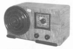
**EMERSON MODEL AX212** – This 1938 radio has a very desirable Ingraham birch cabinet with a green striped inlay. Sometimes referred to as the "Half Mae West Radio," it is a 5-tube set, only 5½" tall and 9" wide. (Wally Worth – Wollaston, MA)
