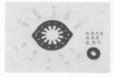
Figure 5. Shown here are the parts required to rebuild a wafer switch. The phenolic stator is located at the center of the figure and is surrounded by the replacement contacts. The ten eylets are shown on the right. Below the eylets is the phenolic rotor.
