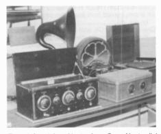
Front, left to right: a Neutrodyne Corp. Neutrodial 3-dial battery set selling at \$60; an Atwater Kent 37 metal box receiver at \$45. Rear, left to right: a Hartford Metal Products Supertone horm speaker at \$150; an Atwater Kent Type E cone speaker, including an RCA 100 speaker, at \$95.
