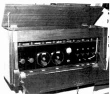
Figure 1. A front view of the 8-tube home brew from the U.S.A.
