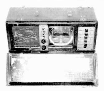
ZENITH MODEL 7G605 — The first of the Trans-Oceanic models, this shortwave receiver is a 7-tube portable with a black leather ettecovered cabinet. It was manufactured in 1941 in two versions, one with a sailboat on the speaker grille, and this one featuring a World War II bomber. (Clark Trissell — Lincoln, NE)
