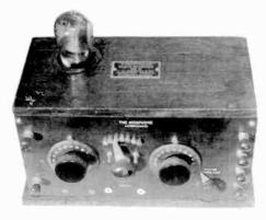
BOWMAN AIROPHONE – Manufactured by A.W. Bowman & Co. of Cambridge, Mass., this 1-tube receiver sold for \$20 in 1922. The tube is inserted through the lid opening, which is not hinged for access. (Merrill Bancroft – Townsend, MA)
