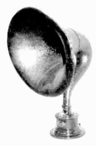
THOMPSON MODEL H-3 – Manufactured by the Thompson Mfg. Co. of Jersey City, New Jersey, this horn speaker has a knob on the base to adjust the sound. (Wally Worth – Wołlaston, MA)
