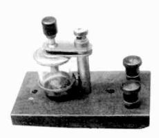
**DEFOREST DETECTOR**—This vertically mounted crystal detector is one of two styles made by De Forest. The other version was mounted horizontally. The wooden base on which it is mounted is not original. (Dave Crocker—Mashpee, MA)
