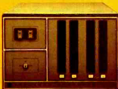
System Three Two to four disks Up to 512K of RAM/ROM Up to 1 megabyte of disk
