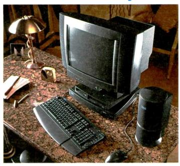
Basic black? Hardly! The Aptiva S series PC looks different because it is. Starting with the "Split Design" that keeps high-demand functions like CD ROM and floppy drive access at your fingertips while moving the PC tower over 6 ft. away—everything about the way this PC works makes more sense. Disk drives are housed in a space-saving console that can be folded down to provide a storage shelf for the keyboard. With the PC off and keyboard stored, you'll have a lot more work surface!
