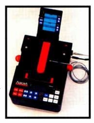
The unit includes a carrying case, battery, charger, cleaver, heat oven for heat-shrink sleeves and an RS232 port for splice data downloading.
