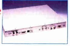
New System Combines Video, Ethernet and T1 A unique new multiplexer, the Series 7000 Supermux will multiplex one baseband video channel, two audio channels, Ethernet, T1 and RS232 data. The product, developed by Radiant Communications, combines information via a high speed TDM system and transmits both ways over one or two fibers for up to 70Km.
