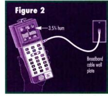
Measuring hum modulation at cable wall plate
