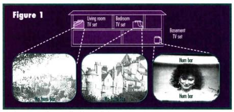
Checking for hum bars on all cable-installed TV sets
