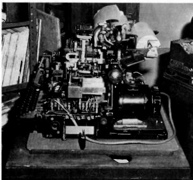
Photo B. The Model 19 printer with cover removed. Note the terminal strips with all the wires going every which way. Don't be intimidated! Only two sets of connections are really necessary, one for the ac and one for the dc loop. See Fig. 1 for loop details. Also note use of 1/4-inch phone plugs for easy changes in equipment location.
