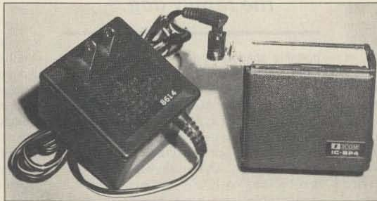
Photo A. The WB9RRR el-cheapo IC-BP4 charger adapter, inserted under the rails of the battery pack. See Figure 1 for foil layout on board bottom.
