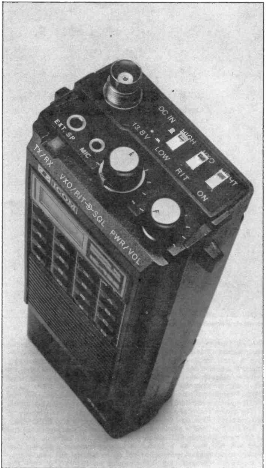
Close-up of the top panel controls — note the RIT control needed for these frequencies
