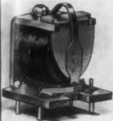
The LR-1301 relay, for printed circuit mounting, has palladium inlay contacts to assure good contact with dry circuit switching. Coil resistances up to 10 K can be had in either treated or un-treated coils. The terminal mounting block can be furnished in either glass epoxy, glass silicone, or phenolic. Overall dimensions are 3/4 in. square by 1/8 in. high; weight, 13 grams.
