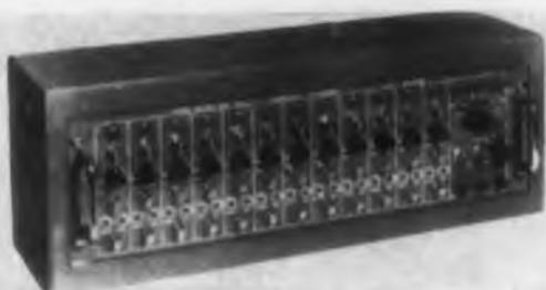
Model 438-B bridge balance unit serves as a bridge between a transducer of one, two, or four-arm type strain gage and a recording oscillograph. It has provisions for completing any part of the bridge circuit not contained in the transducer, and for balancing the bridge and adjusting the sensitivity. Automatic standardization can be accomplished either by series or parallel methods.
