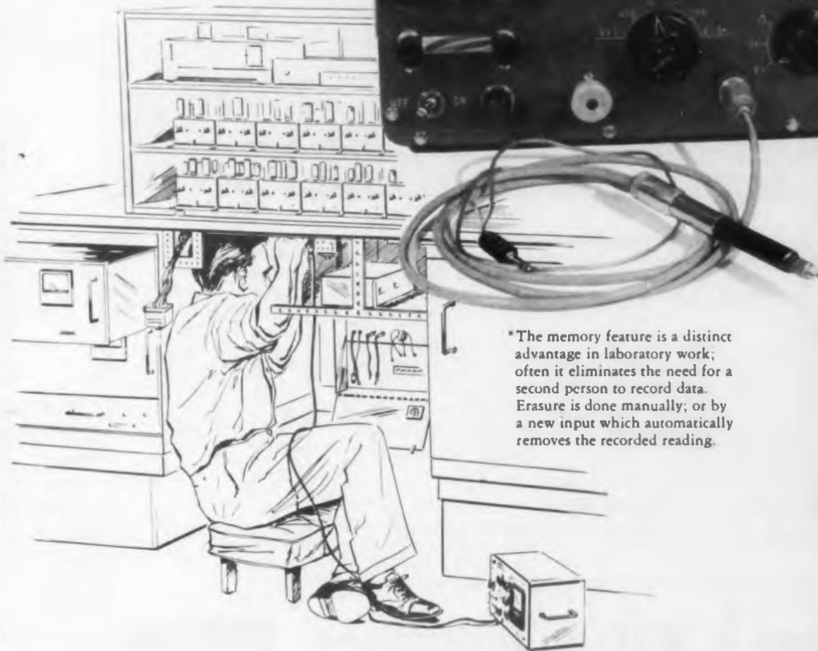
\*The memory feature is a distinct advantage in laboratory work; often it eliminates the need for a second person to record data. Erasure is done manually; or by a new input which automatically removes the recorded reading.
