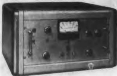
Model C-2910, spectrometer is designed to count only those pulses lying within a selected channel defined by front panel controls, and can provide from 750 to 2000 volts with a regulation of 0.01 per cent of the ac line voltage. Maximum counting rate is 10,000 counts per sec. Five different ranges are provided for both count rate and integral methods of operation.
