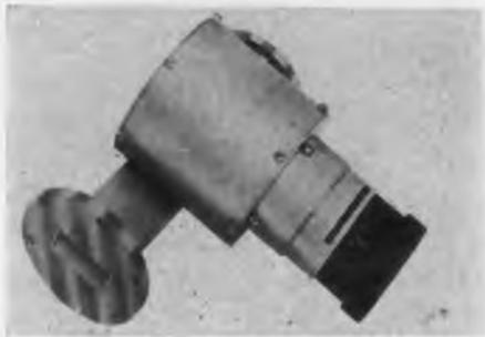
A direct-reading meter, Type 590-A allows quick determination and reading of frequencies between 5100 and 5900 mc. The unit consists of a mode cavity resonator tuned by a non-contacting plunger whose position is variable along the axis of the cavity. The reaction-type meter insures a symmetrical dip over the entire frequency range and therefore eliminates ambiguities.
