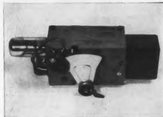
**ELECTR-O-VANE CONTROL UNIT**—A torque of 2 gram-inches or less actuates this precision switch. Use it as a limit switch to operate valves, lights or hopper openings, in response to motion of weighing beams or other members. Use it to sense other mechanical movements—to operate protective devices when a diaphragm is bulged or near rupture, for example.
