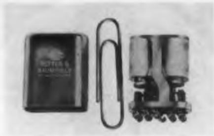
This dual-coil relay, model SL, operates on a 1-w, 3-msec pulse to either coil. A magnetic latch and high contact pressures hold the contacts closed under 100 g shock and 30 g vibrations to 2000 cps. The relay will switch loads up to 2 amp at 30 v dc resistive or 1 amp at 115 v ac resistive, and operates in ambient temperatures from -65 to +125 C.
