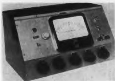
Intended to indicate the percentage deviation of a sample resistor from a standard resistor, type 957 bridge offers very high accuracy over a resistance range from 1 ohm to 10 meg through the use of a chopper-stabilized feedback amplifier. Accuracy as a limit bridge is better than 0.05 per cent for resistances greater than 10 ohms.
