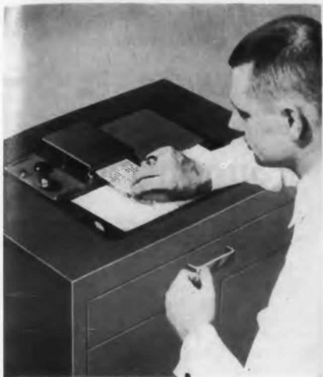
Sliding punched card into the slot actuates the switch. Knob on the left releases it.
