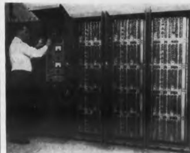
The Addaverter links an analog and digital computer so that both may simultaneously track various phases of missile flight.
