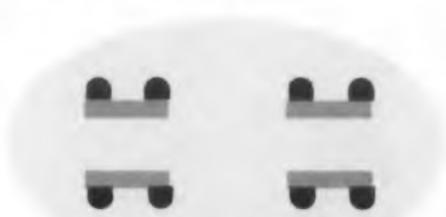
**D** Mica slots are designed with flat alignment surface and channel index to position grids with much greater precision. Closer element spacings are possible where extra Gm is required.
