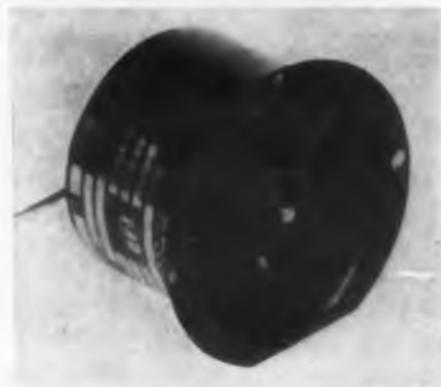
Weighing less than four ounces, this axial blower measures 1-1/2 in. length, 2 in. diam., with a 2-1/2 in. mounting flange. It is single phase, operating on 27.5 v 400 cps or on 115 v 400 cps, and delivers 10 cfm at 0.11 in. static pressure with 5 w input.
