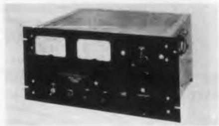
Supplying up to 36 v dc and 15 amp at any voltage, model H3615 transistorized power supply has a combined line and load regulation of less than 0.5 per cent for changes of load from 0-15 amp and for line changes from 105-125 v. Output ripple is 3 mv over most of the range. The instrument measures 8-3/4 x 19 x 14 in. and weighs approximately 50 lb.
