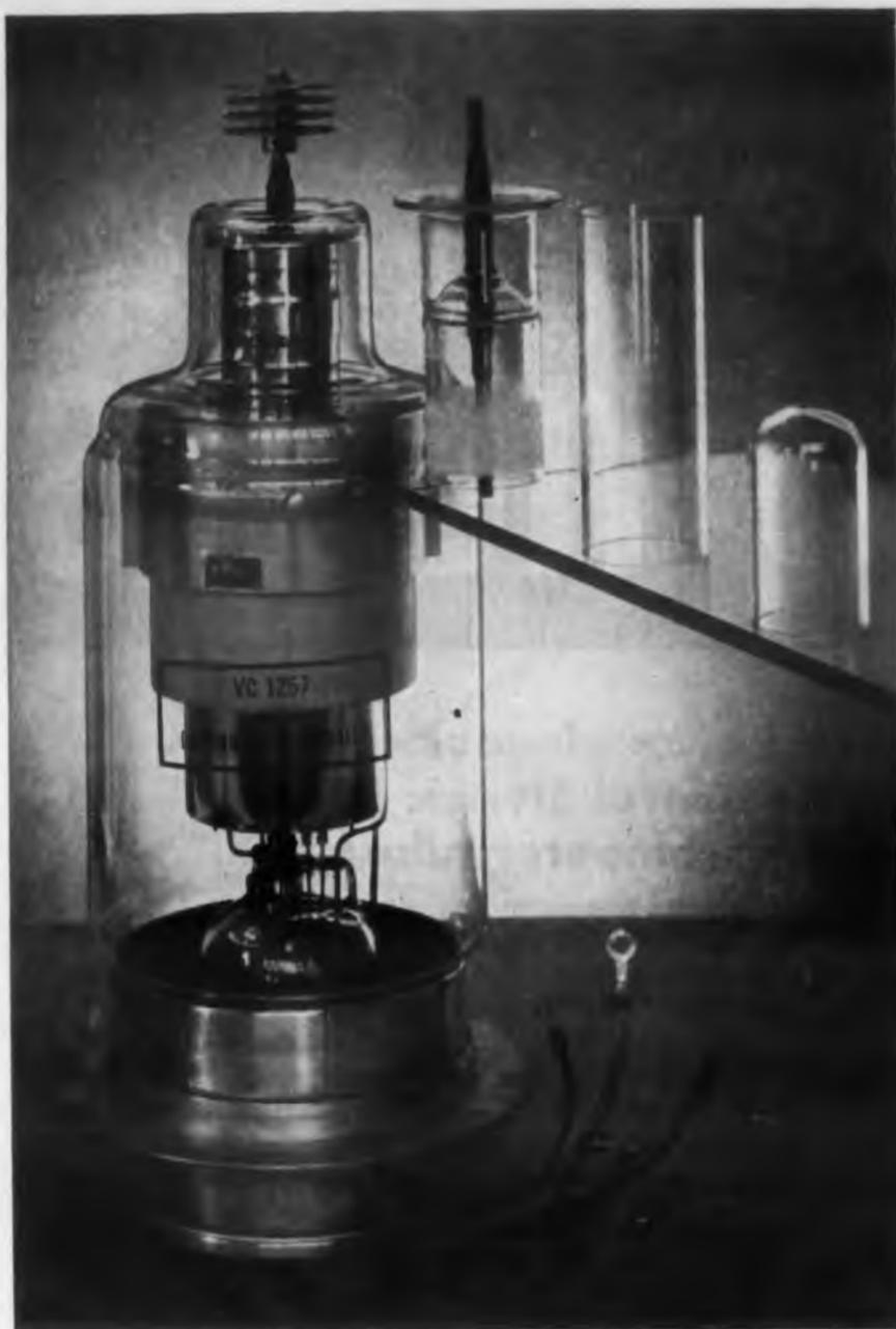
The 33 megawatt hydrogen thyratron shown above is just one of the many special purpose electronic tubes manufactured by Chatham Electronics, a Division of Tung-Sol Electric, Inc. The precision glass components shown in both photos are typical of those supplied by F & P for use in thyratrons and other tube products manufactured by Chatham.
