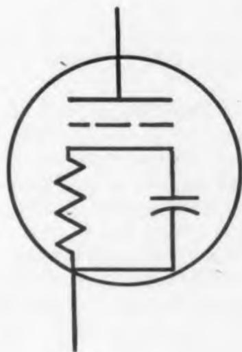
Fig. 14. Tube symbol showing cathode-interference effect, resulting from leaving heaters on standby with plate voltage removed. A "drooping" pulse output results.
