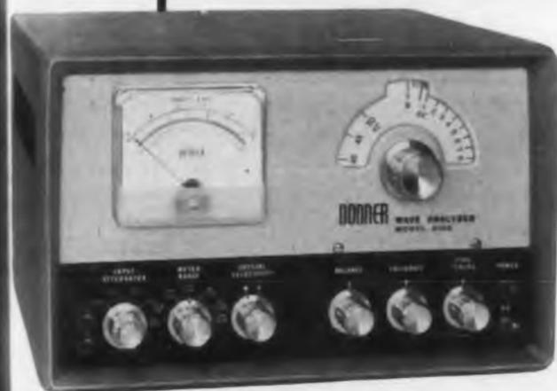
Donner's new Model 2102 Wave Analyzer accurately measures amplitude and frequency for each component of a complex input waveform, whether or not the components are harmonically related. Selectivity, controlled by a front panel switch, provides narrow or wide band pass. Narrow selectivity permits easy separation of input signal components. Broad selectivity permits rapid scanning of the spectrum.
