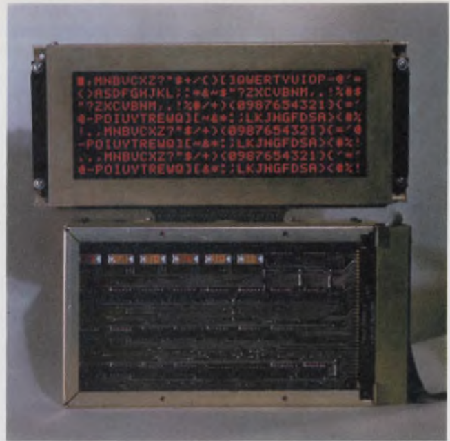
As many as 256 alphanumeric characters can be displayed on Burroughs' Self-Scan gas discharge panel. The panel includes all decode, drive and scan circuitry.
