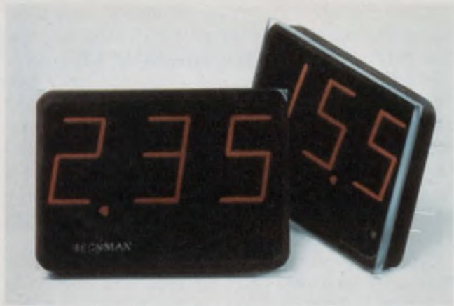
Attractive gas-discharge displays, like this one from Beckman, can be viewed even in direct sunlight. They use high voltage, but need little power.
