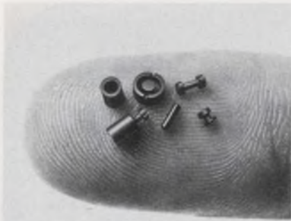
Some of the world's tiniest cores, from TDK Electronics, these are (clockwise from top left): sleeve pot, bobbin, another bobbin, rod, and bobbin slipping into a sleeve.
