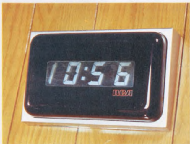
An experimental 2-in.-high, 3-1/2 digit dynamic scattering liquid-crystal readout, designed for digital-clock applications, has been fabricated by RCA.
