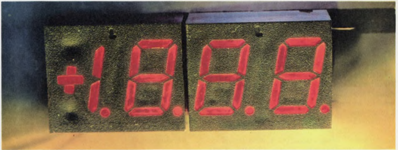
A new trend in large LED displays is to package them as multiple-digit units. The DL 721 and DL 727 from
