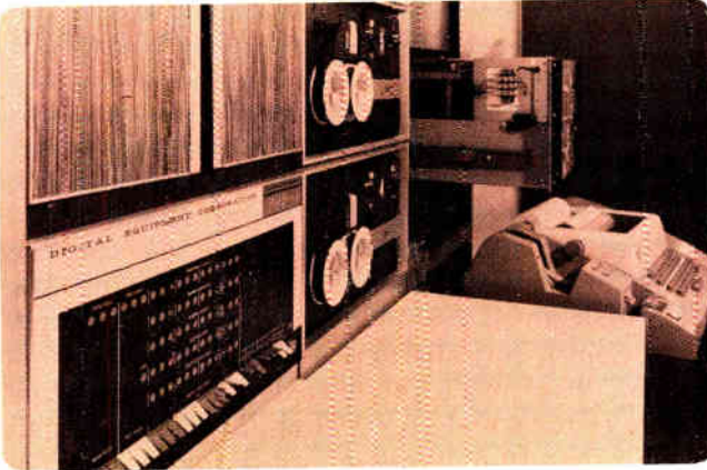
A computer the size of a two-drawer file cabinet, the PDP-8 became popularly known as a minicomputer. When Digital Equipment Corp. offered it in 1965, the mini cost $9000 less than its less powerful and larger predecessor, the PDP-5.
