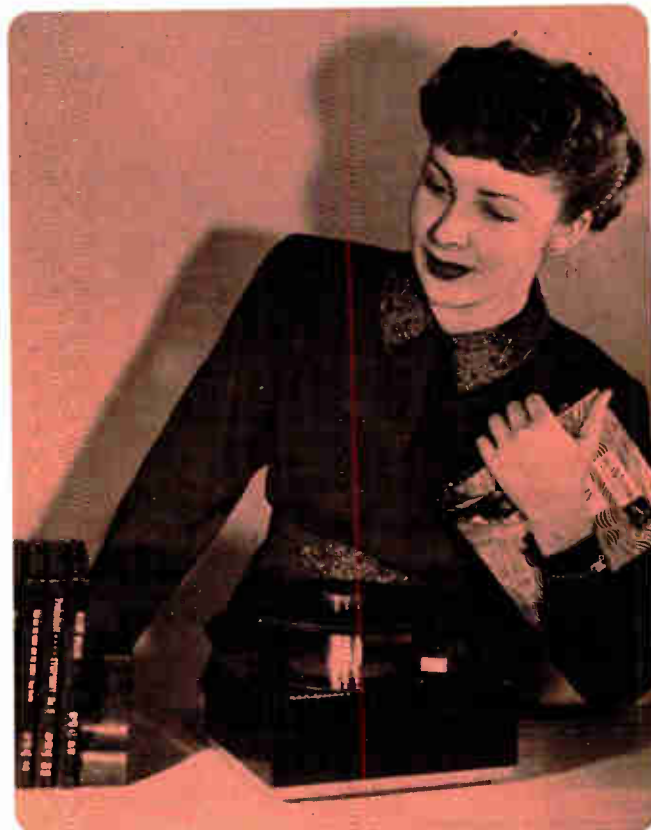
In 1949 the 45-rpm phonograph record was developed by RCA, which also developed a fast record changer that connected to TV sets and played the records through the TV amplifier. Today, the 45-rpm disc is still the "pop" recording medium.
