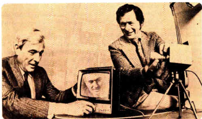
Charge-coupled devices found use in experimental TV camera, demonstrated by Bell Labs' Willard Boyle (left) and George Smith—the inventors who received a patent for charge-coupled devices in 1974.
