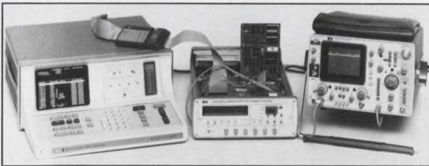
2. Hewlett-Packard's Logic State Analyzer can save much testing time by expressing computer instructions in human-language mnemonics.
