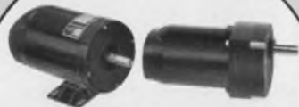
42A Permanent Magnet D-C Motors and Parallel Shaft Gearmotors. Just 4.30" in diameter. Motors TENV 1/8, 1/6, 1/4 Hp. Gearmotors have helical steel gearing.
