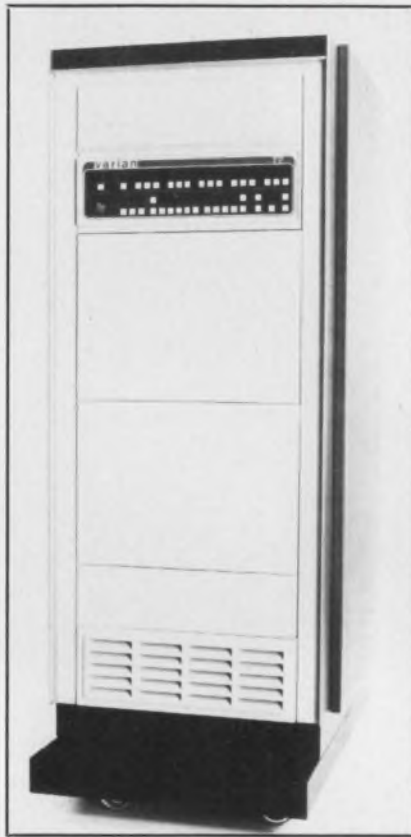
3. The V77-600 is the top of Varian's latest line of minicomputers. It has features originally introduced on large computers, such as user micro-programmability, and a cache-memory. It also uses memory mapping to address one-million 16-bit words.
