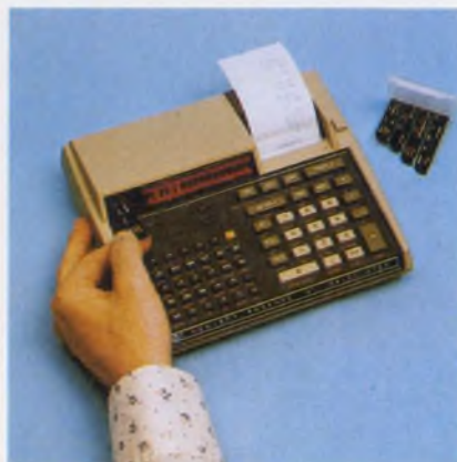
A thermal printer aids programming and debugging in the HP-97 card-programmable machine.
