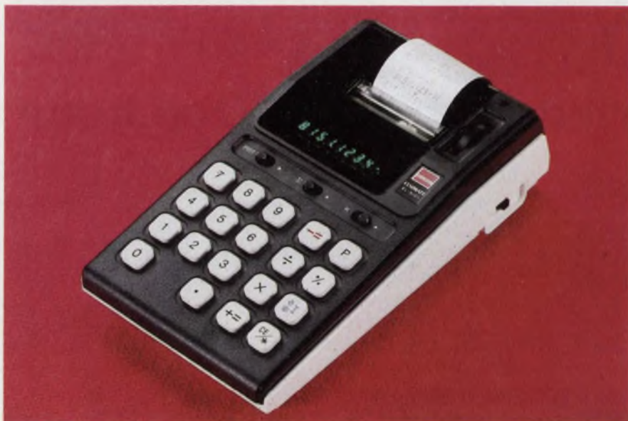
Printers are appearing in hand-held calculators. The electro-sensitive paper in the Sharp EL-8151 responds to voltage impulses from the printer matrix elements. It operates from the unit's NiCd rechargeable batteries.
