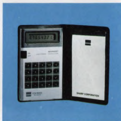
Solar cells keep the batteries continuously charged in these calculators by Royal Typewriter (top) and by Sharp (bottom). These units have liquid-crystal displays and CMOS.
