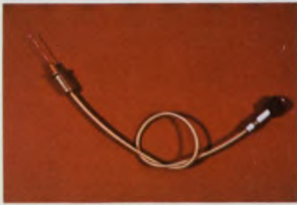
A 660-nm LED is mated with a section of DuPont single-channel plastic fiber-optics cable in this pigtail assembly by Aborn Electronics.
