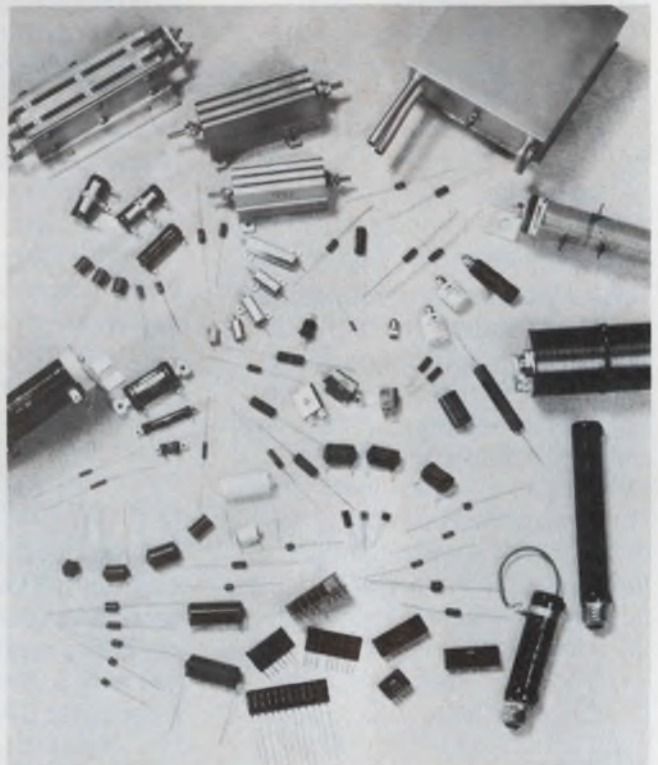
1. Wirewound precision and power resistors come in a large variety of body sizes and shapes. Axial, radial, PC-mounting and multilead-network types are all available as precision units. And power units often have ceramic bodies, through-tab mounting and vitreous coatings. Special units come with lamp bases or water cooling.
