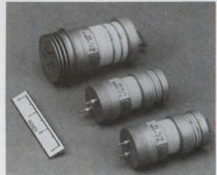
Unpackaged EBS devices from Watkins-Johnson are video amplifiers. The middle tube has 750-V, 7-A peak output.
