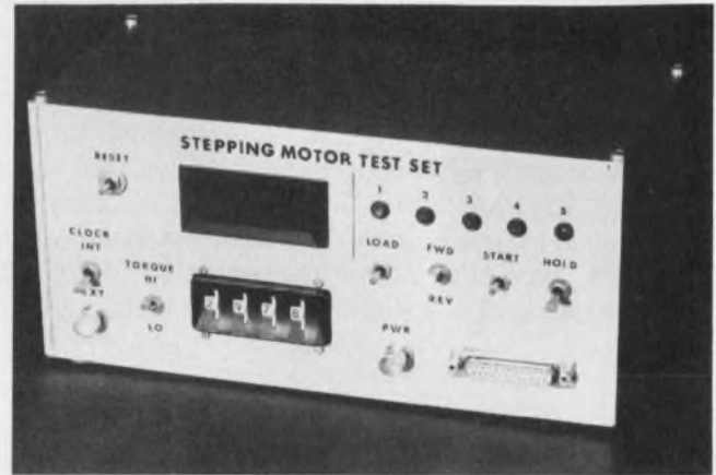
1. Building a stepping-motor tester like this one gives you a convenient method for breadboard testing before constructing production hardware.
