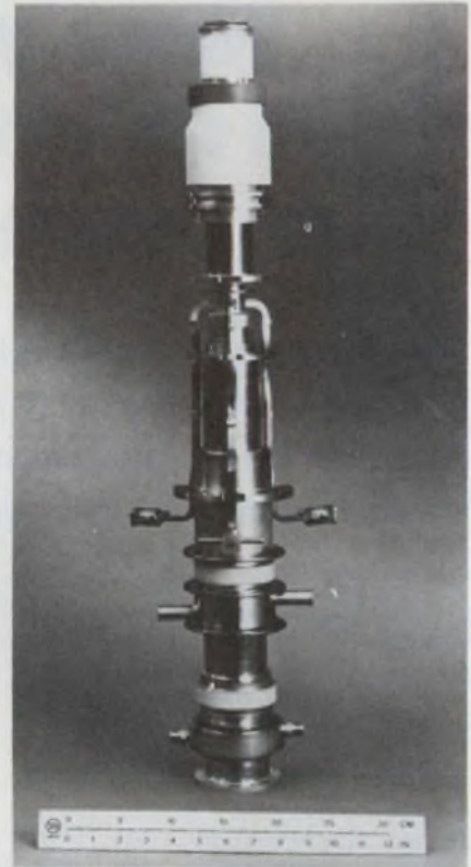
Experimental pulsed gyroklystron amplifier is used for plasma heating at 28 GHz. The rf output is at bottom.
