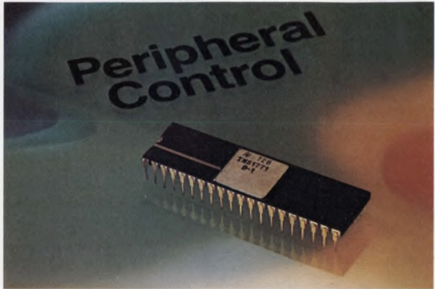
Microprocessor companion chips are simplifying the short-haul data-communications link between \mu Ps and their system peripherals. This is National Semiconductor's INS-1771, a floppy-disc controller-on-a-chip.
