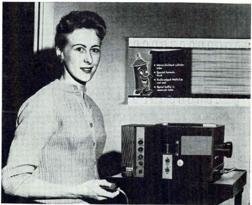
Stripfilm picture and optically recorded sound track message (inset) are projected and reproduced in synchronism by Kalart Co. still projector
