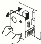
Get quick replacement/ accessibility of plug-in chassis by simple half-turn of handle.
