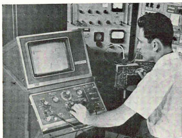
ITT sampling oscilloscope being used to test power conversion module of Ranger spacecraft
