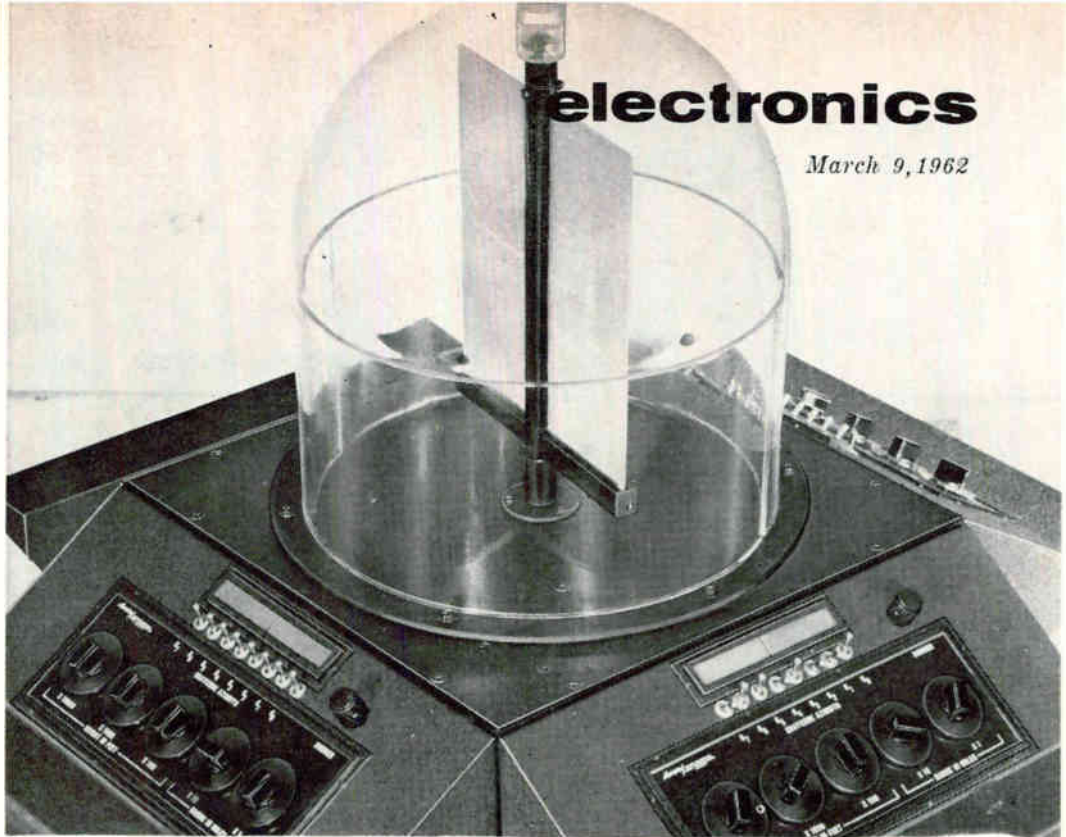
Three-dimensional solid-state display showing rotating electroluminescent panel and three target consoles for simulation display (Avco)
