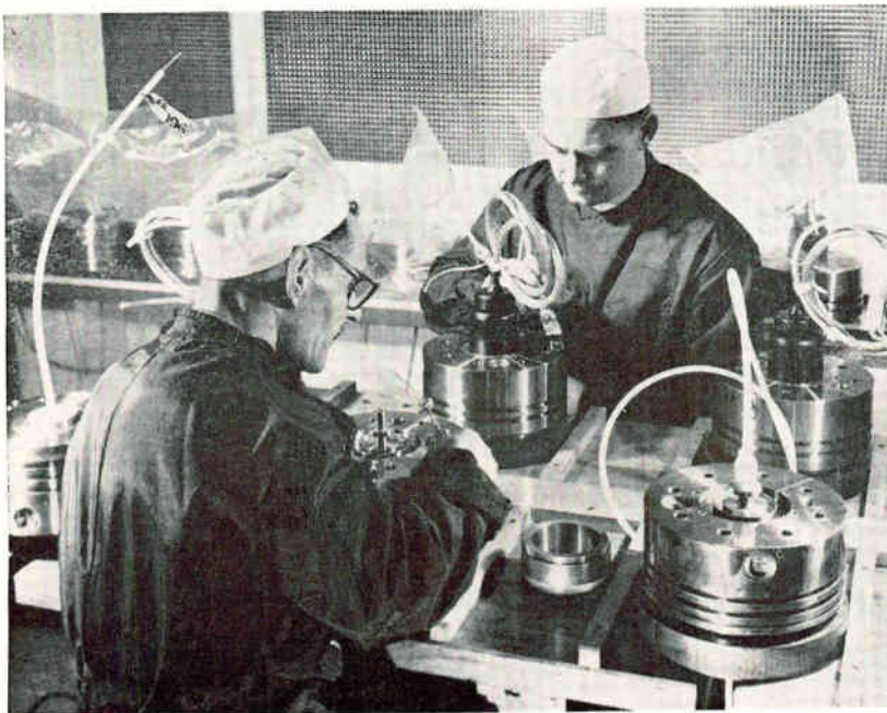
THE FRONT COVER. Bulkheads to protect submerged telephone repeaters from high pressures of the Atlantic Ocean bed are inspected at Standard Telephone and Cables, Ltd., British affiliate of I.T.T. Gold plating on major inside metallic surfaces reduces possibility of metallic whisker growth that could cause short circuits during long untended life
