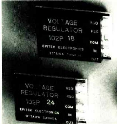
w. Specifications include regulation of 20 mV for load current of 0 to 1.5 A; 10 mV per volt input change, and temperature coefficient of 0.01%/°C. Epitek Electronics Ltd., 19 Grenfell Cres., Ottawa 12, Ontario, Canada [385]
