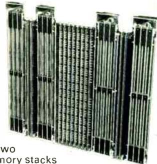
Here's a real eye-opener for computer designers—Toko's new 65K byte memory system, HS-400L. It's constructed with two basic sub-assemblies—woven-plated-wire memory stacks and electronics packages. Designed for medium and large scale computers, the HS-400L offers high reliability, easy maintenance and a flexible arrangement of word lengths.
