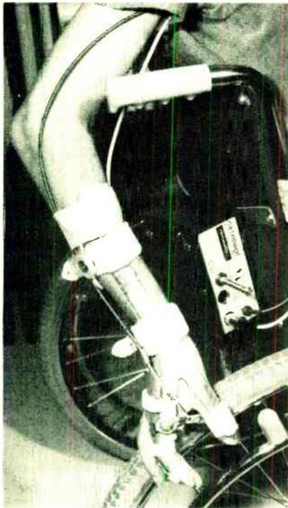
**Gripping.** Unit uses impulses from single muscle for holding, tightening, or releasing.
