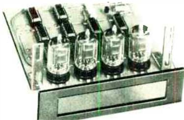
plays do not appear blurred. The modules operate from a single 5-v source, are available with three to six digits complete with TTL-compatible latches, driver-decoders, and decimal point at each position. Price is \$20 per digit. Tronix Inc., Box 349, Phillipsburg, N.J. [384]
