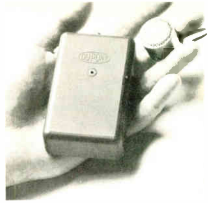
Quiet touch. DuPont calls its wearable noise-measuring device an audio dosimeter.
