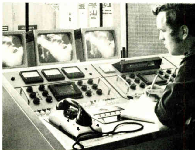
Czech TV. Test color telecasts are to begin this year from tower (above) equipped by Tesla and already operating atop Mt. Ještěd. Inside, transmitter controls (below) are in electronically neutral zone.
