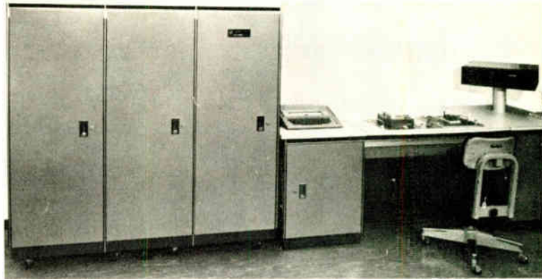
2. Typical system. This example of ATS-960 is in use at TI to test electronic assemblies for radar and other equipment. Test station (console at right) contains test head, indicators, switches, and a data terminal; other equipment is below station and in three racks at left.
