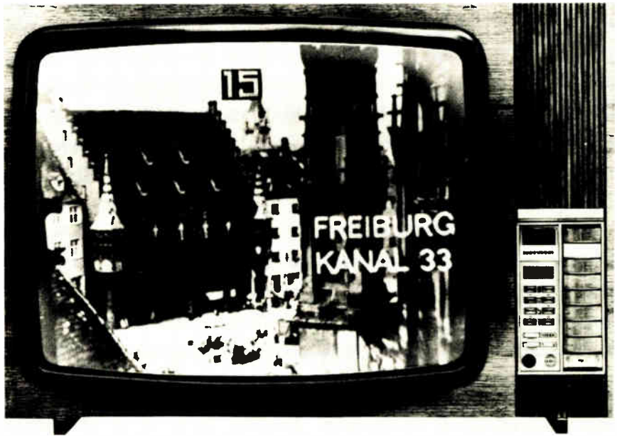
6. Channel 15. The channel display for double-digit numbers is a 2-by-7 dot matrix against a dark 4-by-9-dot background. Each dot is made up of six TV-line sections, each 0.4 microsecond in duration.
