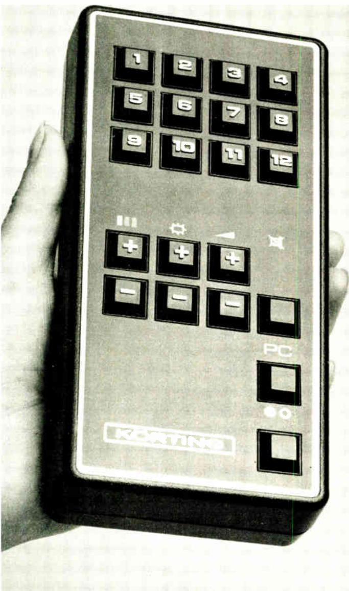
1. Remote connection. A recent use of MOS technology for television receivers is the hand-held ultrasonic transmitter unit designed for remote control of channel selection, picture tuning, and volume control. This unit can handle up to 30 commands if needed.
