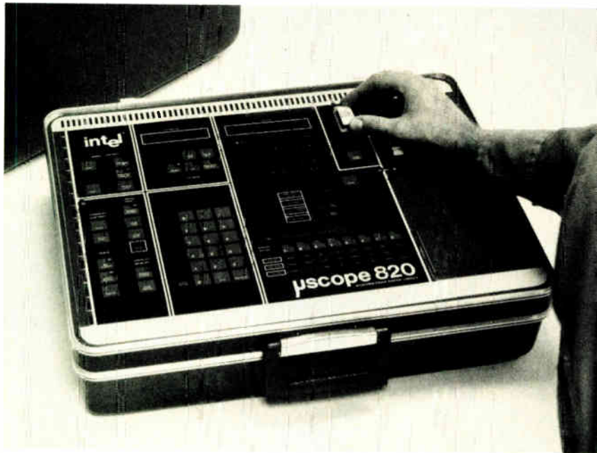
Speed. To use \mu -Scope to test any microcomputer-based system, service personnel need only remove the microprocessor from its socket and insert the \mu -Probe connector in its place.
