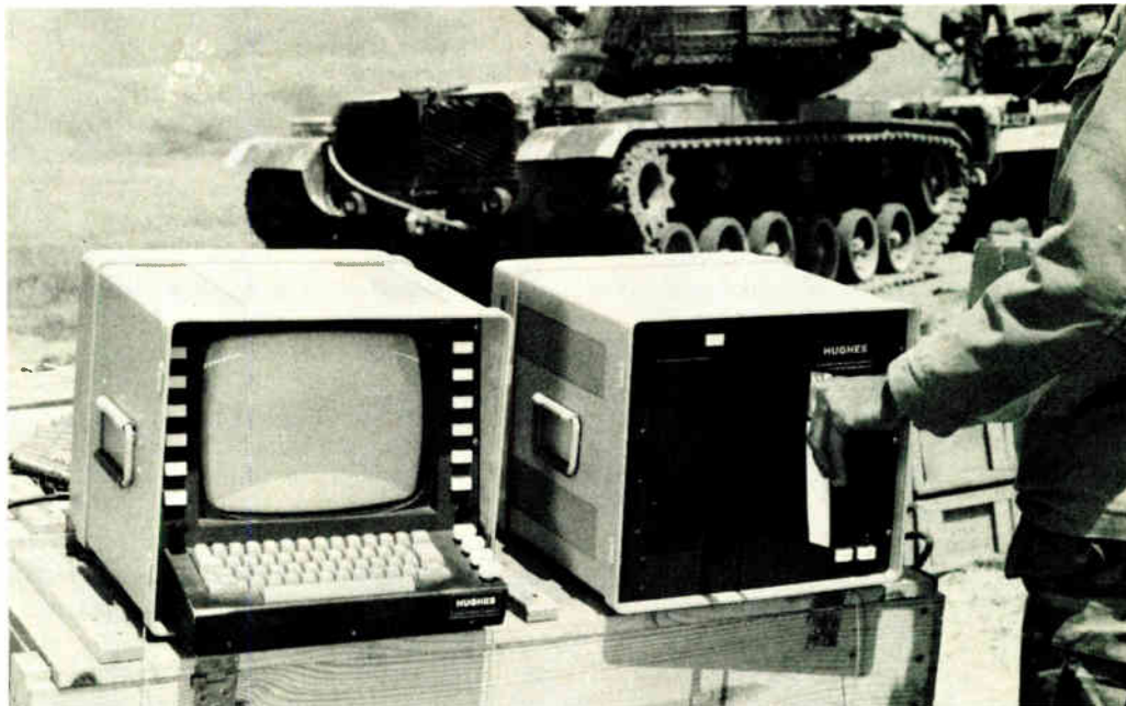
On the go. With Hughes-built microprocessor-based repair system, faults in complex electronic gear can be diagnosed in the field by relatively unskilled technicians.
