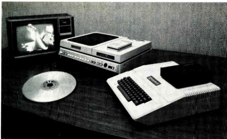
Tie-in. Discovision Associates will offer a system, with either an RS-232 or IEEE-488 link, that puts a laser video disk player under computer control, making the player a storage peripheral.
