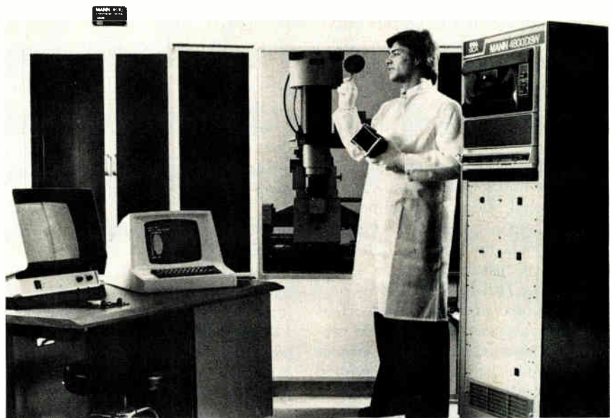
Head start. GCA Corp.'s Mann 4800 DSW wafer stepper is the only model that is operating on a significant number of production lines. But other makers are rushing into the market.
