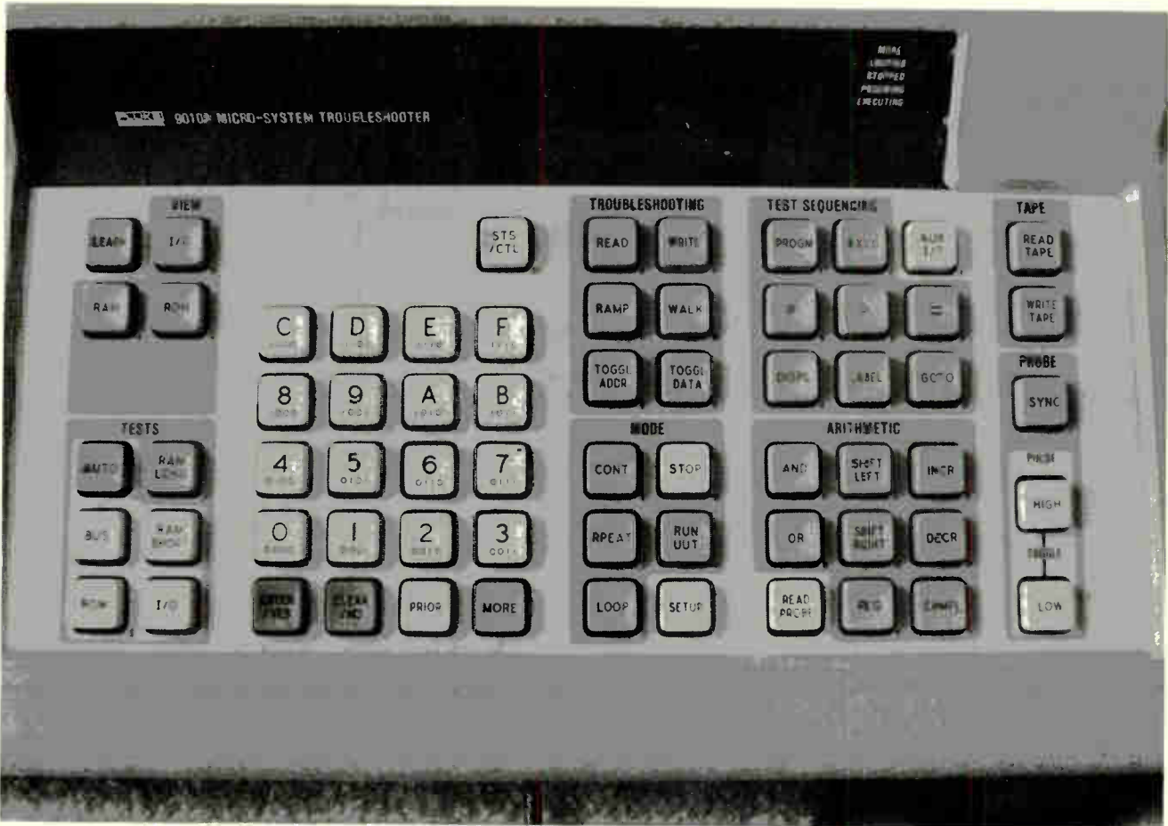
2. User interface. The instrument's keyboard is laid out in a clear and highly functional manner, so that it takes little time to become familiar with it. The learn, view, and test keys (left) allow a user to start checking a board in minutes with the displayed operating mode (right).
