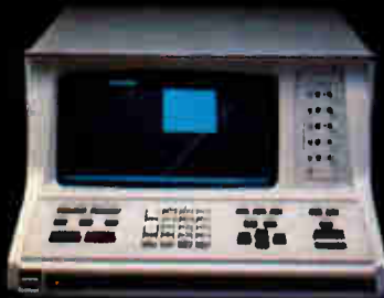
Hewlett-Packard 1610B A sophisticated data-domain-only logic analyzer
