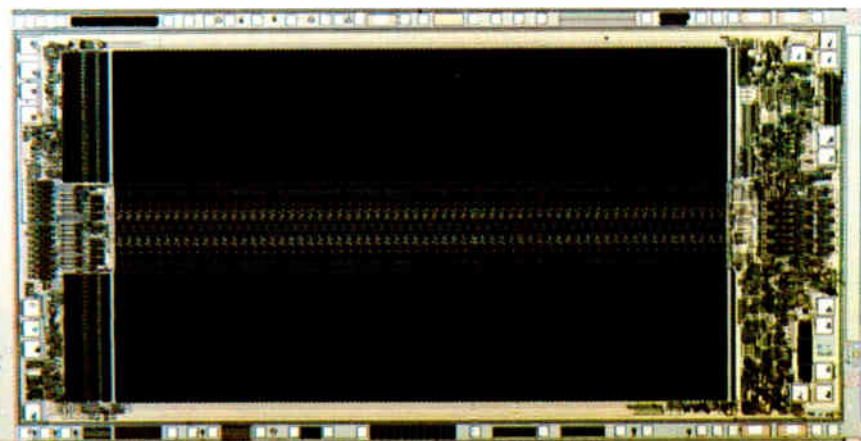
TI's new TMS4416 16K x 4 DRAM uses advanced design concepts developed for TI's pacesetter TMS4164 64K DRAM. For example, square array architecture results in less power dissipation, lower junction temperatures, greater reliability, and lower cost.
