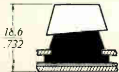
Actual size cutaway of low-profile actuator module
