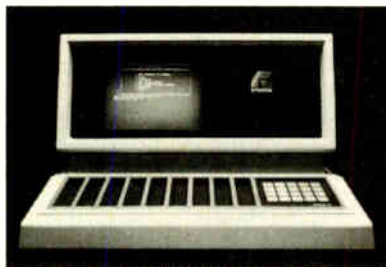
On the spot. With a new programming terminal designed for use at retail outlets, customers can have new game software downloaded from a mainframe into reusable E-PROM-based cartridges for Atari, Commodore, or TI personal computers.
