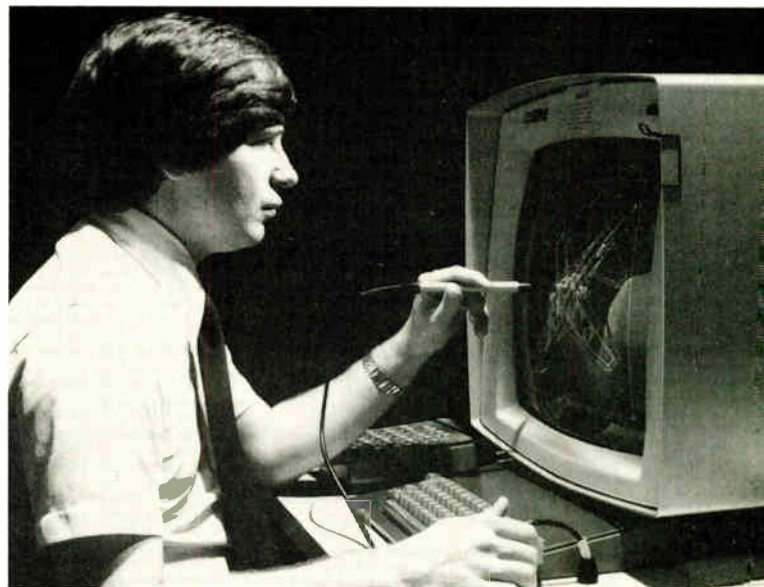
More than a drafting aid. Computer-aided-design (CAD) work stations are taking the drudgery out of many design tasks through the use of interactive graphics displays and an extensive data base.
