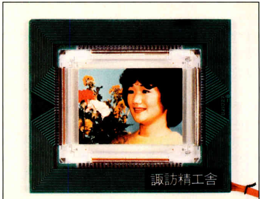
Color sandwich. Tiny color TV receiver includes liquid-crystal cells sandwiched between polarizers. The lower substrate carries the FET array and pixel electrodes with individual red, green, or blue filters above each. Four IC drivers, each capable of handling 120 gate or data lines, are distributed around the display's periphery. Photo shows actual size of device.
