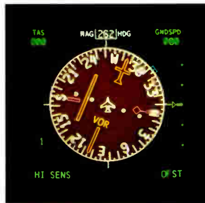
The first electronic horizontal situation indicator to eliminate the vertical element of a curved screen.
