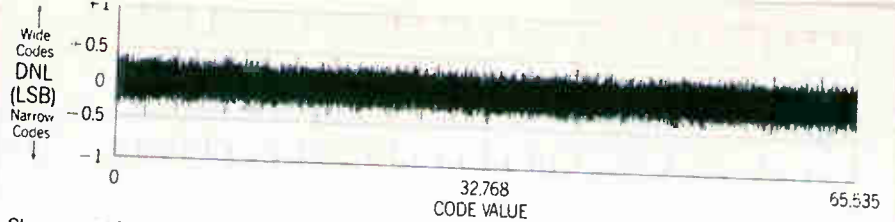
Shows < \pm 0.7 LSB code width variation from ideal (definitely no missed codes)
