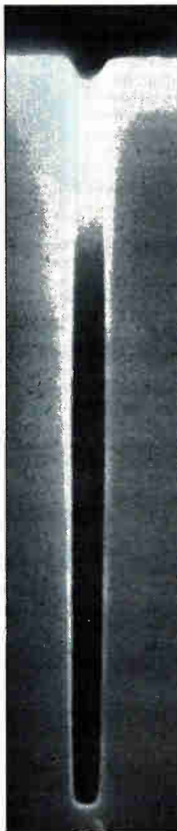
The trench, with its 21:1 aspect ratio, in 0.2-by-4.2- \mu\text{m} , is etched into single-crystal silicon.
