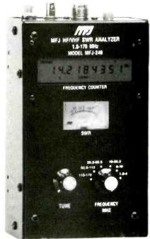
Figure 1: MFJ-249 SWR Analyzer
