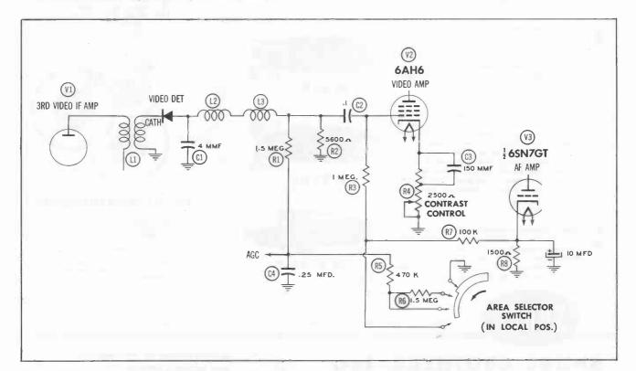
Figure 3. Partial Schematic Showing Area Selector Switch.
