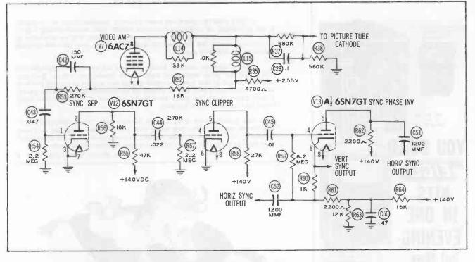
Figure 6-7. Triode Sync Separator Plus Sync Clipper and Phase Inverter.
