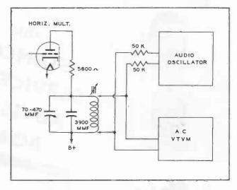
Figure 7. Setup for Checking Ringing Coil.
