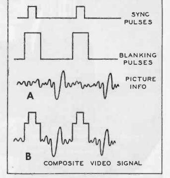
Figure 5-1. The Composition of a Video Signal.
