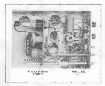
Figure 2. Photograph of Adjustable Horizontal Output Transformer and Centering Control.
