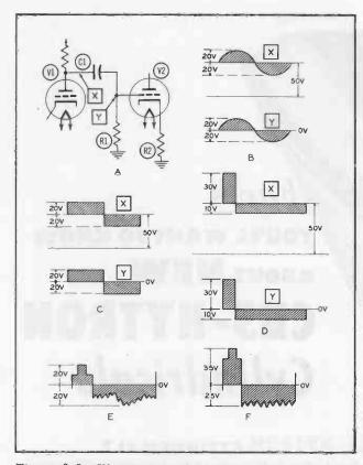
Figure 6-3. Illustrations Showing how the AC Axis of a Signal Varies in Position.
