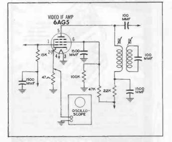
Figure 2. Setup for Tracing Hum with Oscilloscope.
