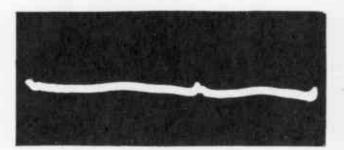
Figure 4. Waveform at W1; Receiver Operating Normally with AGC Clamped.
