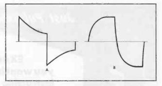
Figure 10. Distortion of Square Wave Caused by (A) Poor Low Frequency Response; and (B) Poor High Frequency Response.
