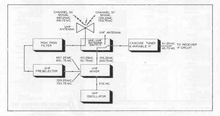
Figure 5. Block Diagram Showing Function of Tuner Circuits for Two Available UHF Signals.
