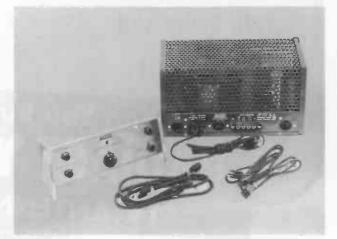
Figure 1. A-333-A Amplifier and A-433-A Preamplifier.
