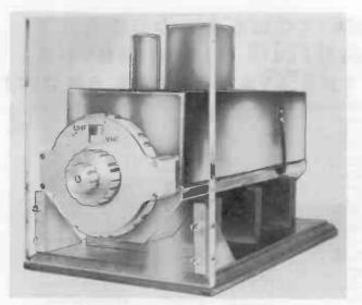
Figure 4. Tuner Mounted to Show Control Knobs in Place.
