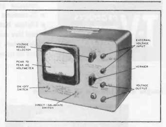
Figure 8. Hickok Model 630 Television Voltage Calibrator.
