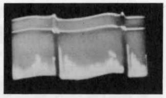
Figure 2. Waveform at Video Detector Load (W6); Receiver Operating Normally.
