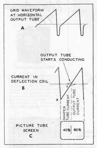
Figure 2. The Various Current and Voltage Relationships in the Horizontal Deflection Output Circuit.
