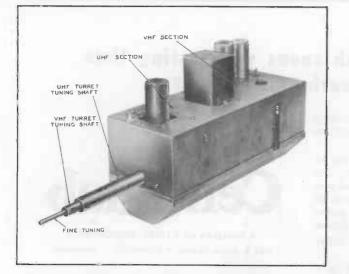
Figure 1. Standard Coil 82 Channel Turret Tuner.
