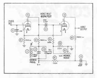
Figure 3. Horizontal Multivibrator with Ringing Coil.
