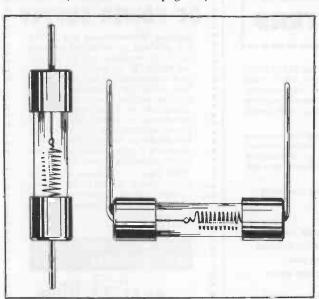
Figure 4. Glass Tube Fuses with Pigtails.
