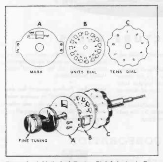
Figure 3. A Method of Tuning Dial Indexing to Provide VHF or UHF Channel Selection.
