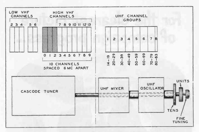
Figure 2. Block Diagram Illustrating a Scheme for Channel Selection.
