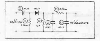
Figure 3. Detector Probe for Use with Oscilloscope.
