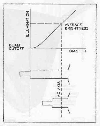
Figure 6-4. The Effect on Picture Tube Illumination by Two Signals Having a Fixed AC Axis.
