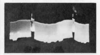
Figure 9. Waveform at W4; Horizontal Output Plate Coupled by Gimmick to Grid of 1st Video IF.
