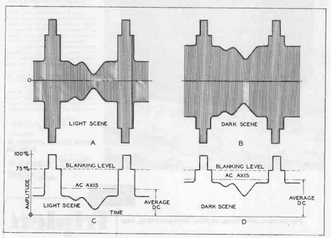
Figure 6-1. Waveforms of Two Signals Representing Dark and Light Scenes.
