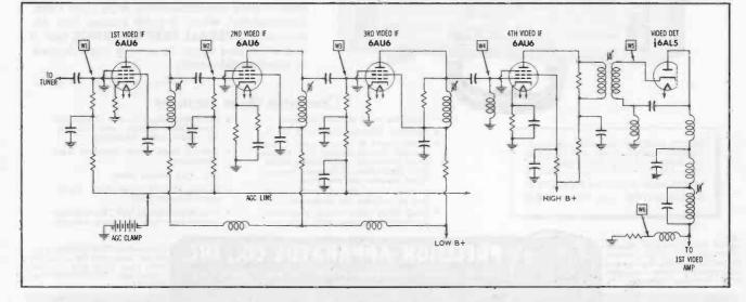
Figure 1. Typical Video IF Amplifier Section with Video Detector. Method of AGC Clamping is Shown.
