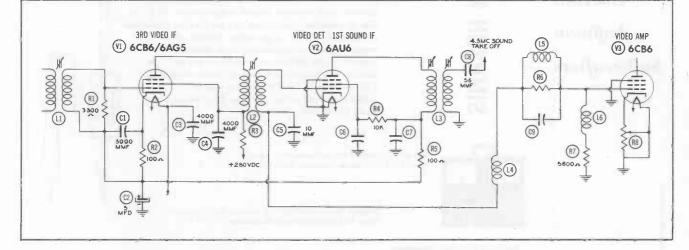
Figure 1. Combined Video and First Sound IF Stage.
