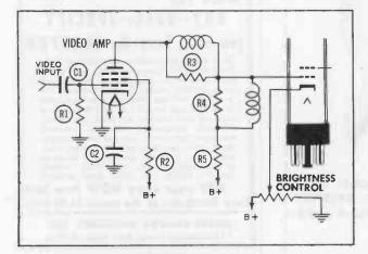
Figure 6-6. Grid Leak Bias Type of DC Restorer.
