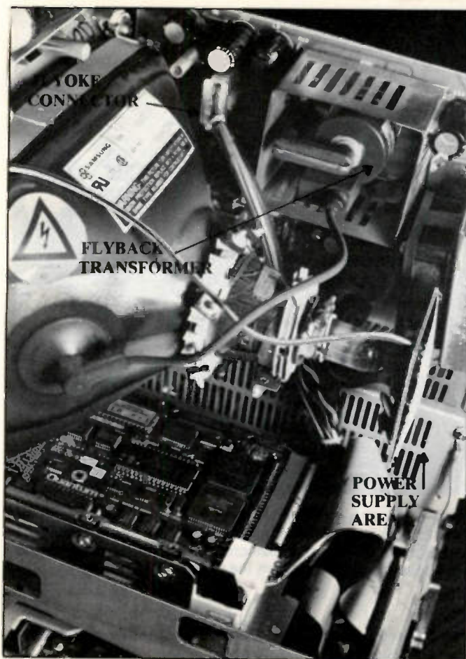
Figure 3. Once you have opened up the Macintosh, this is what you'll find inside. Note the locations of the flyback transformer and the J1 yoke connector.
