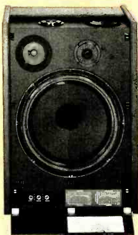
H.H. Scott Pro-100 also reflects sound from ceiling.
