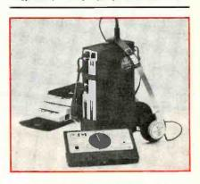
DNR (Dynamic Noise Reduction) is the major feature of Technidyne's model 140 Hip Pocket Stereo. DNR, a low-pass filter system whose cutoff frequency varies with program content, is said by the manufacturer to rid the program source of noise, as well as to prevent noise from being added by the playback equipment. In the model
