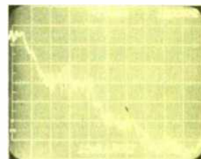
The 20-kHz swept audio shows dropping off at 8 kHz (2 kHz/div.)
