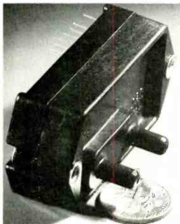
Fig. 3. A solid-state pressure-to-current transducer (149PC) made by Honeywell's Micro Switch Div.
