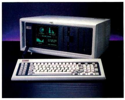
The Compaq Plus includes a 10M-byte hard disk and 9" monitor.
