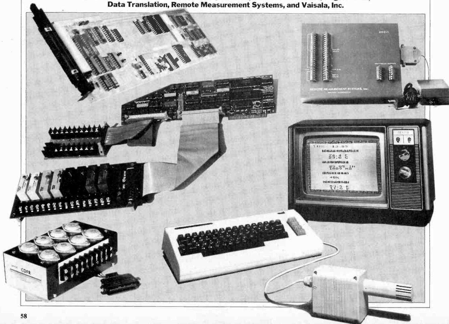
Clockwise from lower left are data acquisition systems from Vantec, Rogers Labs, Data Translation, Remote Measurement Systems, and Vaisala, Inc.
