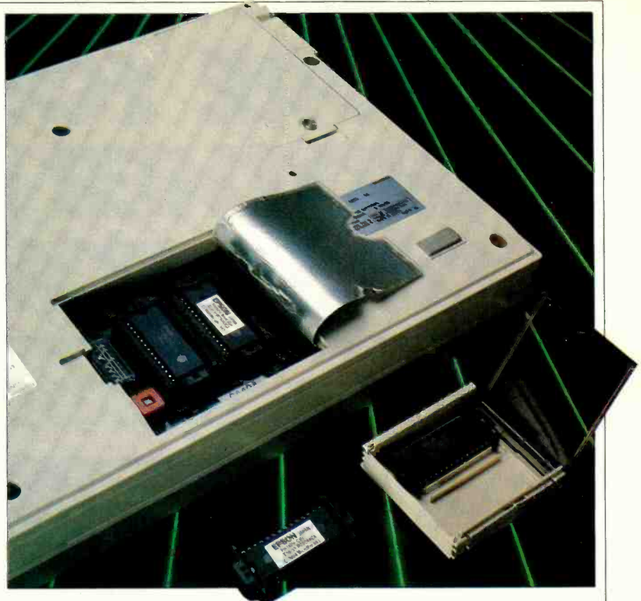
ROM modules for the PX-8 can be inserted and removed by the user.
