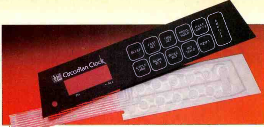
Fig. 5. Membrane keypad with legend overlay.
