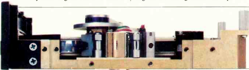
A side view of the self-threading Interdyne drive.
