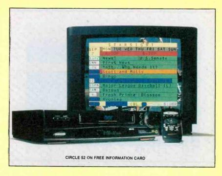
Besides the remote control layout, the main differences between using a Star-Sight-equipped VCR and a stand-alone unit are in the initial hookup and in recording programs. Instead of the double infrared remote emitter supplied with the stand-alone unit, the VR8905 comes with a "cable box mouse"—a fancy name for a mouse-shaped infrared remote emitter used to transmit remote signals from the VCR to the cable box.
