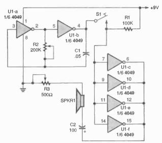
Fig. 5. This versatile code-practice oscillator is great for use by individuals or small groups wishing to learn Morse code. Note that switch SI is a telegraph-type Morse-code key.
