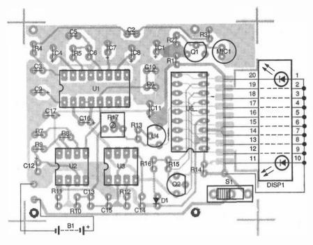
Fig. 4. When installing components to the PC board, use this parts-placement diagram as a guide. The LED display, DISP1, is mounted sideways, off board. The row of pins not connected to pads are connected together by a wire that is then soldered to the pad shown.
