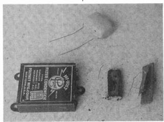
The old 1-µF capacitor (bottom center) as removed from its case (bottom left) and paraffin embedment. A new orange drop capacitor (above) will be installed in the case and wired to the original terminal board (bottom right).
