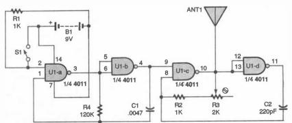
Fig. 1. This is the schematic for the Poor-Man's Transmitter. The circuit gets its name because of the extremely low parts count (and the low prices of those parts).
