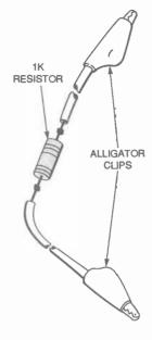
Fig. 3. You should always discharge electrolytic capacitors before fiddling with a circuit. This little tool allows you to do that quickly and safely for moderate-sized units.
