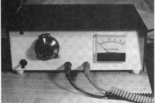
Here's "The Crusher," a variable voltage, high-current supply that can come in handy when testing or using ham gear.
