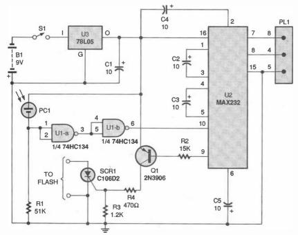
Fig. 2. This is the schematic for the Flash-Battery Tester. A MAX232 (U2) and a 9-pin D plug (PLI) provide a simple interface to a PC.
