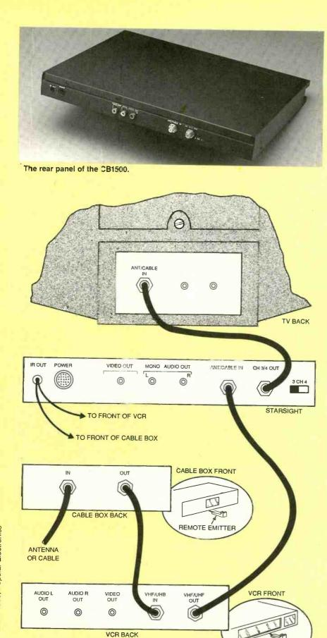
FIG. 2. The typical StarSight setup in volves a TV, VCR, and cable box.
