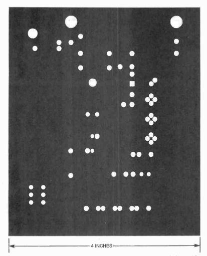
Fig. 4. Here's the component side of the board; it's really just a ground plane with circular etched areas.
