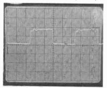
Fig. 5. This shot shows the waveform of the voltage at the output of gate U1-c. which is part of the Transmitter's RF oscillator.
