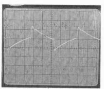
Fig. 4. Here's the waveform of the voltage appearing across capacitor C1. The curving sloping region occurs when CI is keeping gates UI-a and UI-b from switching between two states (see text).
