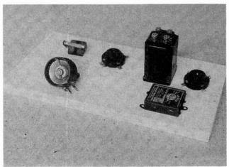
The basic parts were placed on a "breadboard" to check the layout. The board has been ripped down to a 7-inch width (10 inches had been specified) for a more compact parts arrangement.
