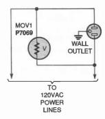
Fig. 2. Placing an MOV across an electrical outlet's terminals is a good way to protect any device you plug
