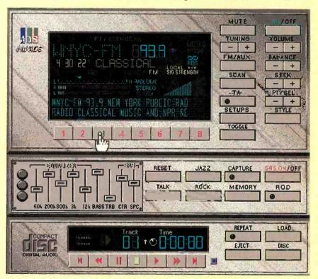
The main Radio Rock-It display—when it works—shows an abundance of information including the call sign, frequency, format, signal strength, and volume level. The station can also choose to send a 64-character message. Many receivers will show such messages as scrolling displays. As you can see here, the ADS attempt to break the message into two lines creates awkward word wraps, and the loss of characters.
