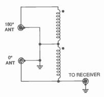
Fig. 7. This phase-shift transformer, based on the 4:1 BALUN circuit, overcomes the transmission-line problems associated with feeding two antennas out-of-phase.
