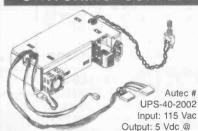
3 amps, 12 Vdc @ 2 amps (4.5 amps peak). 7" X 4.25" X 2.16" metal enclosure with cooling fan. EMI filtered input module, fuse holder, on/off switch, LED socket and two 4 pin power connectors.
