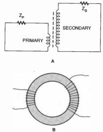
Fig. 2. A basic step-up (or step-down if reversed) transformer is shown in A, while B shows how such a transformer could be wound on a toroidal form.
