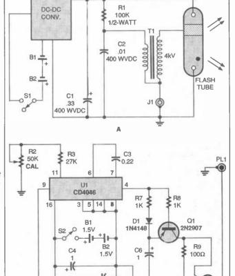
Fig. 4. If you retrofit a flash unit as described in A, it can accept signals from the circuit in B to operate as a precision stroboscope.
