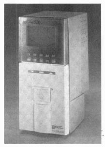
Shown here is a Practical Peripherals 28,800 bps PM288LCD stand-alone modem, which makes use of the fastest speed available over conventional telephone lines.
