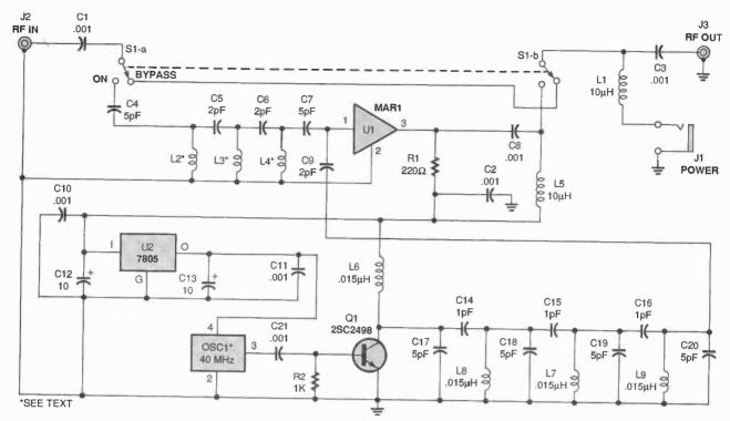
Fig. 2. At the heart of the Converter circuit is OSCI, a 40-MHz oscillator module. Only the 10th harmonic at 400 MHz is presented to the input of UI.
