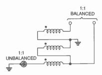
Fig. 6. A 1:1 BALUN requires a trifilar winding; that is, three coils wound together in parallel.
