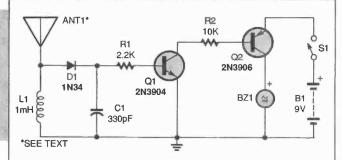
Fig. 4. With the modifications shown here, the field-strength meter makes a great tuning monitor for QRP (low-power) use.
