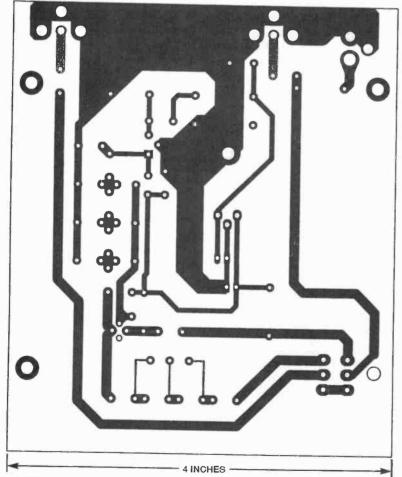
Fig. 3. This is the solder side of the double-sided board. Three of the components, L2–L4, are stripline parts that are etched into the board.
