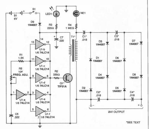
Fig. 1. This circuit uses a transformer to generate a high-voltage output (up to 20,000 volts) from iust four C-cells.
