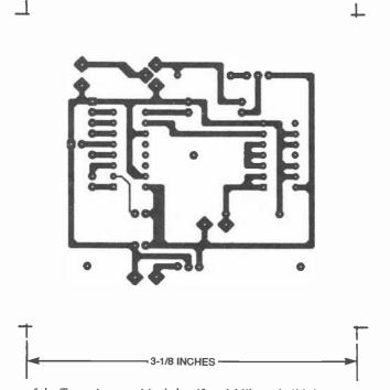
Fig. 3. Layout of the Tester is not critical, but if you'd like to build the project on a PC board, use this template to etch your own.
