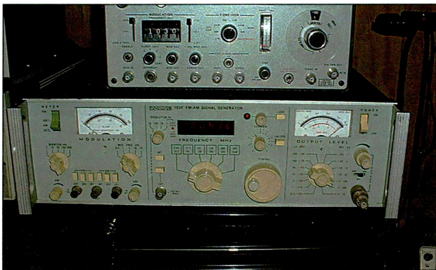
The Boonton 102F is a fine all-purpose lab generator that features digital frequency readout and low phase noise. The generator can be phase-locked to prevent drift. It's a nice unit, but overkill for vintage radio servicing!
