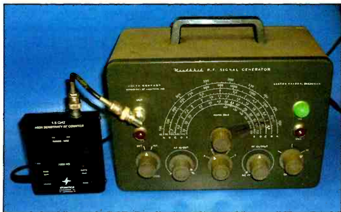
The Heathkit SG-8 and companion StarTek counter. The counter indicates the generator is set to 1600 kHz.
