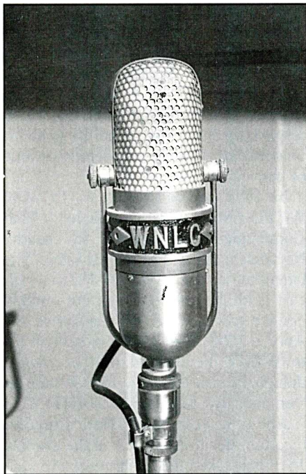
An RCA DX-77 ribbon mic with a rare WNLC center "flag" ring. It hails from the 1490-kc era.
