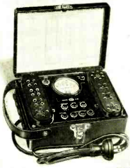
The Franklin tube checker.
