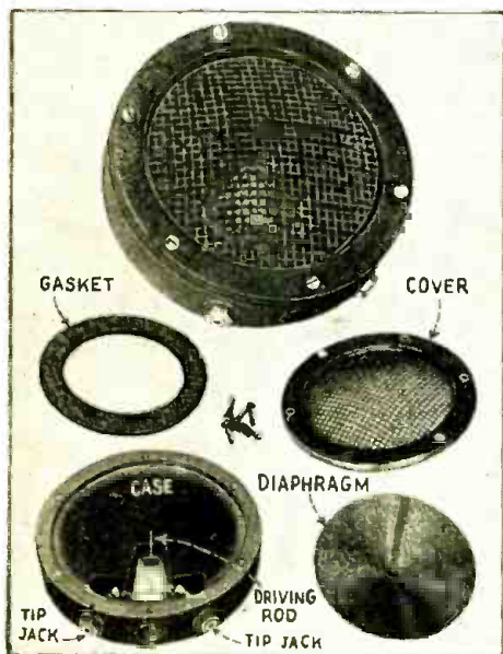
Above is a completely assembled, and below a dismantled view of the crystal microphone.
