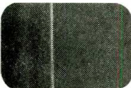
Fig. 5—Line caused by poor linearity.
