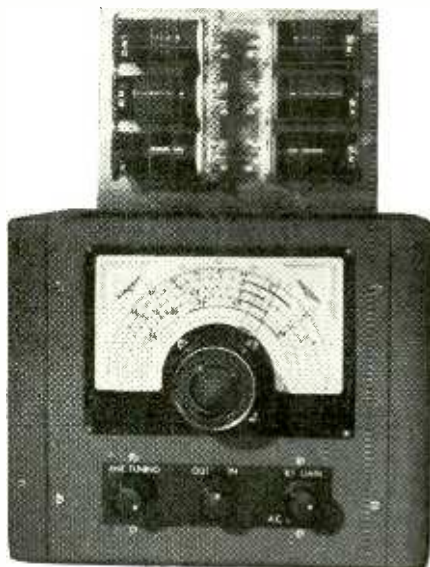
Completed preselector and plug-in coils.
