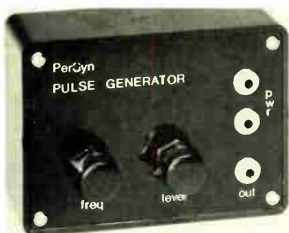
THE PULSE GENERATOR is designed to trigger the PerSyn generator at 1 to 500 Hz.
