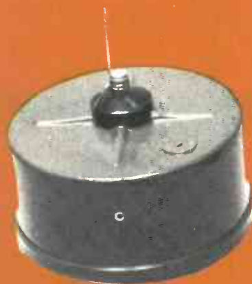
FIG. 7—A COMMON SEWING NEEDLE is used as the electron-emission source. The blunt end of the needle is soldered to the anode of the rectifier.
