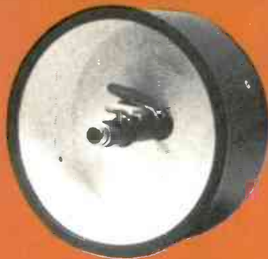
FIG. 6—INTERIOR VIEW of the top PVC cap. Rectifier D1 and capacitors C4, C5, and C6 are shown.
