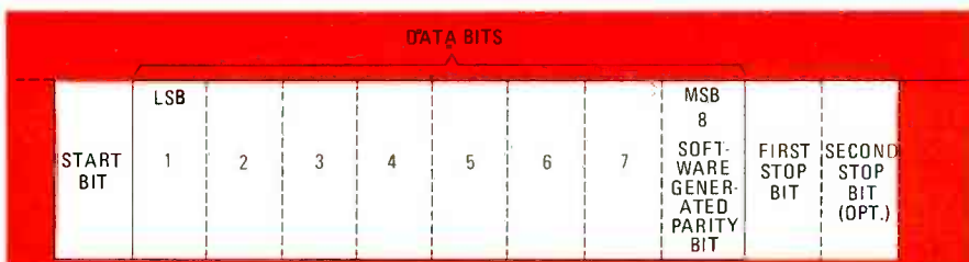
FIG. 14—DATA BITS are transmitted one-after-the-other in serial communications. Note that framing and parity bits are added.
