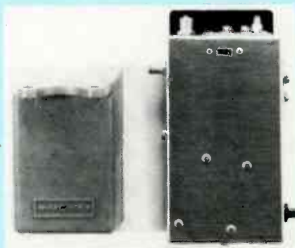
THE OUTPUT IMPEDANCE of this Archer model 15-1134 from Radio Shack, a division of Tandy Corporation, is switch selectable (75 or 300 ohms).
