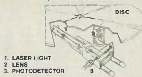
FIG. 4—THE VLP VIDEODISC PLAYER was the first consumer device to use a laser. The three main parts of the system are shown here.
