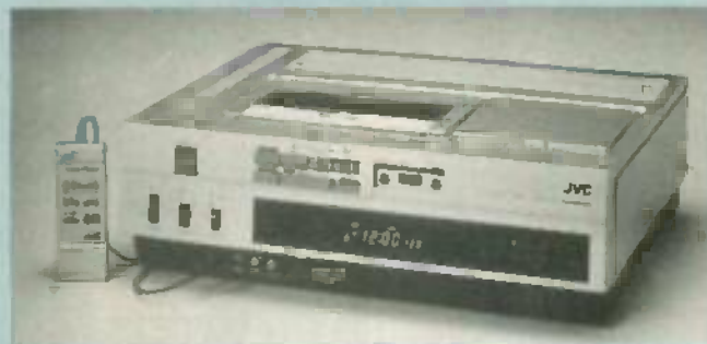
FIG. 13—FOUR HEADS ARE USED in JVC's HR-7300-U. One set is used in two-hour mode, the other in six-hour mode.
