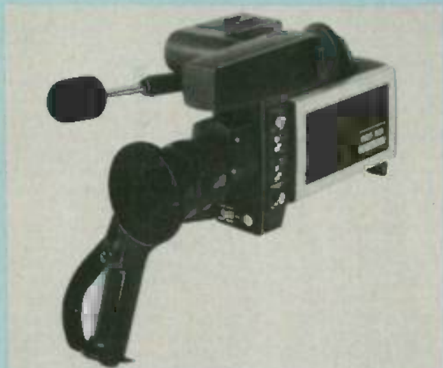
FIG. 2—ONE OF THE FEATURES of the model CC011 color camera from RCA is its sensitivity in low light. It has a minimum light requirement of just 5 foot-candles.
