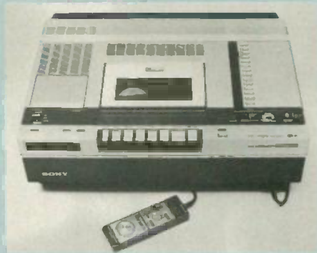
FIG. 12—SONY's SL-5800 uses a double-azimuth head to provide noise-free slow and freeze motion.
