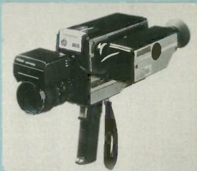
FIG. 4—A TOP-OF-THE-LINE video camera, this model IK-1850AF from Toshiba features a movable electronic viewfinder and an auto-focus system.
