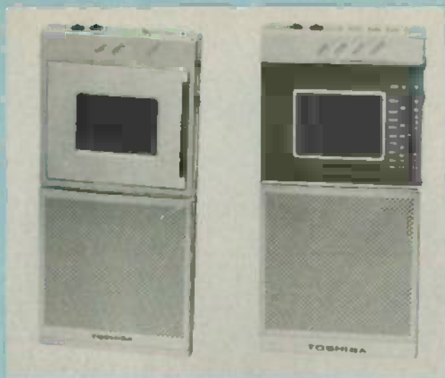
FIG. 3—THESE HAND-HELD televisions from Toshiba use two-inch diagonal flat-panel LCD displays.
