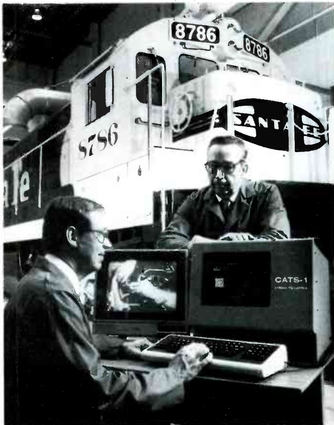
CATS-1, GE'S NEW COMPUTERIZED TROUBLESHOOTER that makes the inexperienced locomotive mechanic into an expert. It can ask questions, diagnose problems, show detailed drawings of the locomotive's components (screen at right), and even demonstrate repair procedures on a video monitor (screen at left). Francis S. Lynch, head of the team that devised the software program, is seated before the instrument; David Smith, whose expertise was tapped to supply the computer with its body of knowledge, stands behind it.
