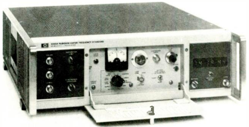
FIG. 5—A RUBIDIUM-VAPOR FREQUENCY STANDARD. This device is manufactured by Hewlett Packard.
