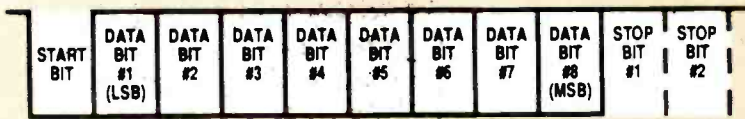
FIG. 3—MOST RS-232 SERIAL COMMUNICATIONS use this older "teletype" asynchronous code. Seven or eight data bits are normally used, with the least-significant bit always sent first. Any number of stop bits above the minimum can be sent between successive characters.
