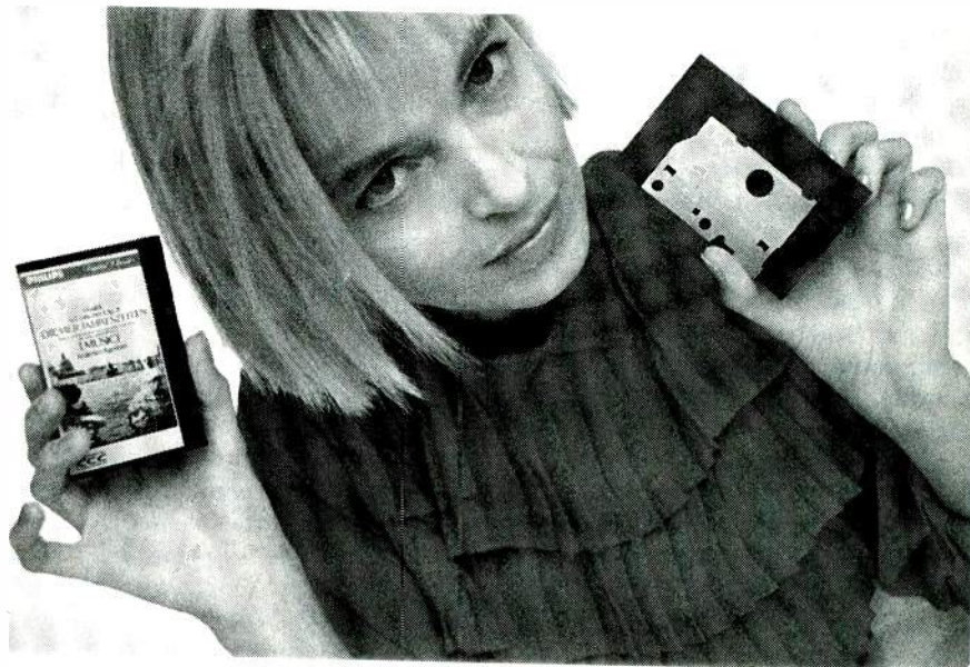
THE NEW PHILIPS DIGITAL CASSETTES will deliver CD-quality sound in a player that is compatible with standard cassettes.
